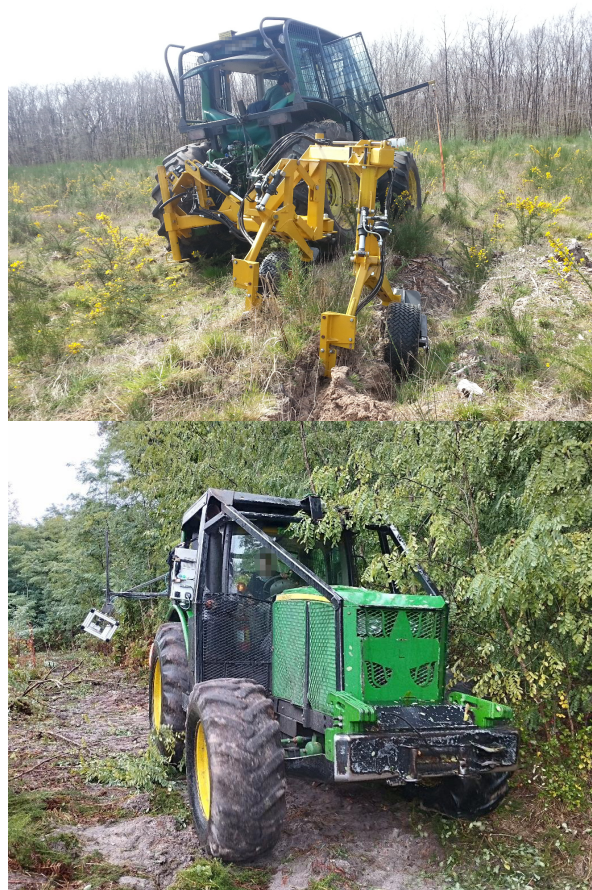
Fig. 1. Top: Typical existing tractor with retractable cutting tool. Bottom: Ruggedized acquisition system attached to a tractor for data collection.
