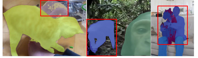
Fig. 7. Some incorrect mask predictions. The erroneous regions, which either overlap or extend beyond the boundaries, are highlighted within the red boxes. In the first two images, there are overlaps between target mask annotations and extensions beyond the respective gtbbox for other targets. In the last image, two target mask annotations overlap.
