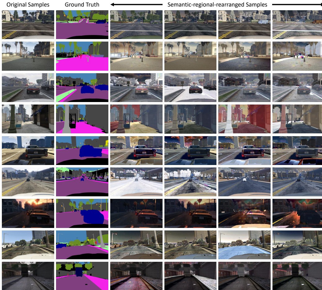
Figure A2: Visualization of semantic-regional-rearranged samples. These samples are obtained from GTAV. The randomized images shown above are reconstructed from the rearranged shallow features via a decoder used only for visualization.
