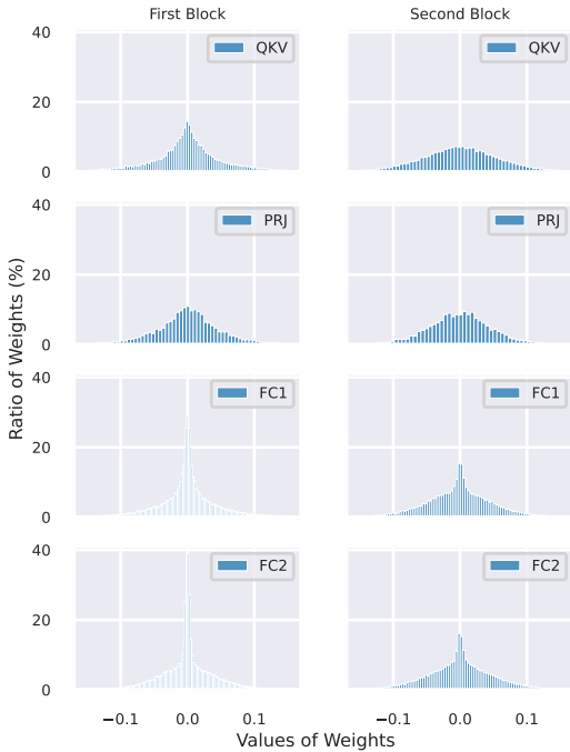
Figure 2: Weight distributions for different functional layers for the first and second Swin Transformer block. The meaning of QKV, PRJ, FC1 and FC2 can be found in Figure 3. The x-axis indicates the values of the weights, and the y-axis denotes the ratios of weights.
