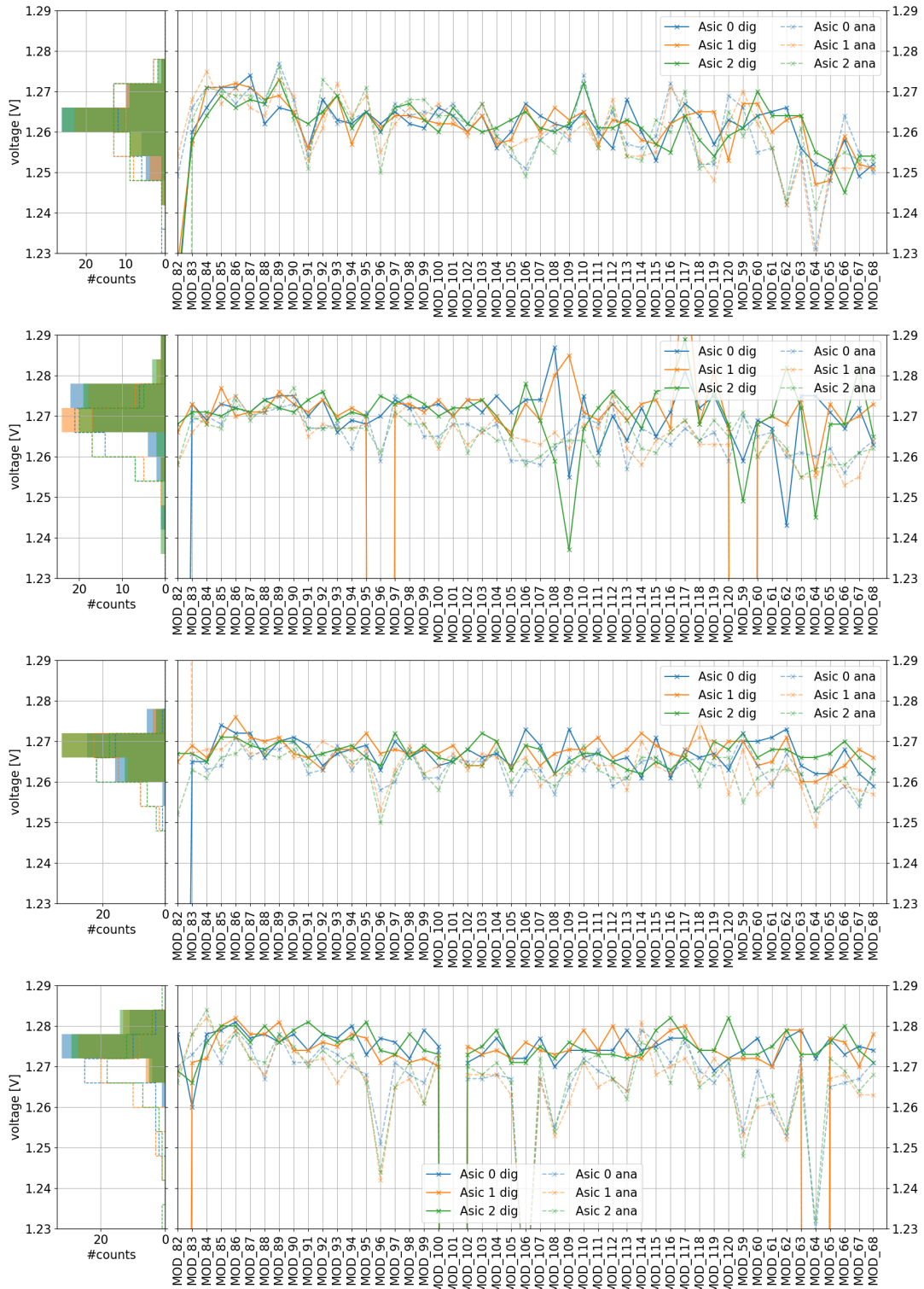
Figure 61: The analogue and digital currents, measured by the VeloPix chips, as a function of module number across the production. The plots are for the four tiles on each module, arranged from top to bottom as CLI, CSO, NLO, NSI. In each plot the analogue and digital voltages of each of the three ASICs is shown.
