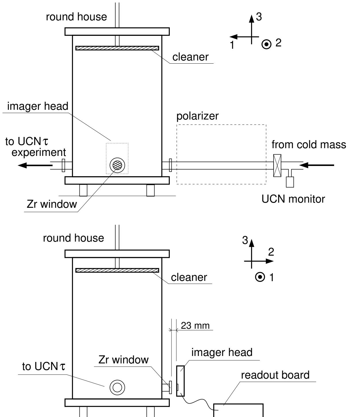
Figure 2: Experimental setup for detection tests. UCNs from the cold mass was filled in a buffer volume, referred to as the round house. Cleaner was positioned select UCNs with energy around 100 neV. The imager was positioned 23 mm away from the Zr window. Direction 1 corresponds to the direction toward the UCN $\tau$  experiment[11, 12], while direction 2 is to this imager test. Direction 3 indicates the vertical axis.
