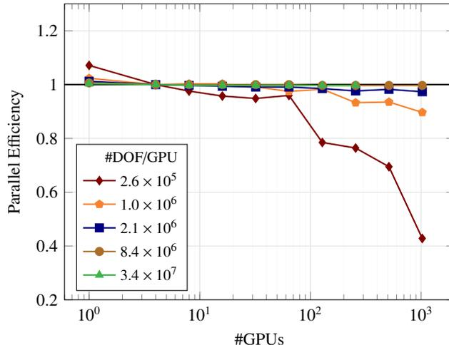
Figure 7: Weak scaling of GALÆXI with the split-form DG scheme and  $N = 7$  plotted as the parallel efficiency over the number of GPUs for specific loads, i.e. DOF per GPU. The parallel efficiency is computed based on the PID on a single node, i.e. on 4 GPUs.
