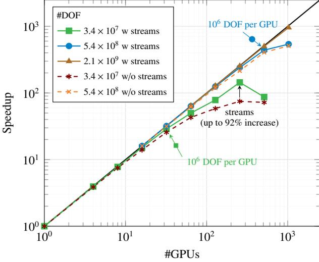
Figure 8: Strong scaling of GALÆXI with the split-form DG scheme and  $N = 7$  plotted as the speedup over the number of GPUs for three problem sizes. For two cases, the results without the use of parallel streams are shown dashed. The speedup is computed based on the smallest number of GPUs that was able to run the given case. The ideal speedup is shown in black.
