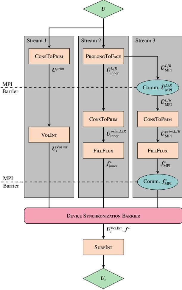
Figure 4: Flowchart of GALÆXI for a single evaluation of the convective DG operator using streams. Some routines comprise several individual compute kernels instead of single, monolithic device kernels. These are summarized here to keep the flowchart concise. Moreover, the lifting procedure to compute the gradients is omitted here for readability.
