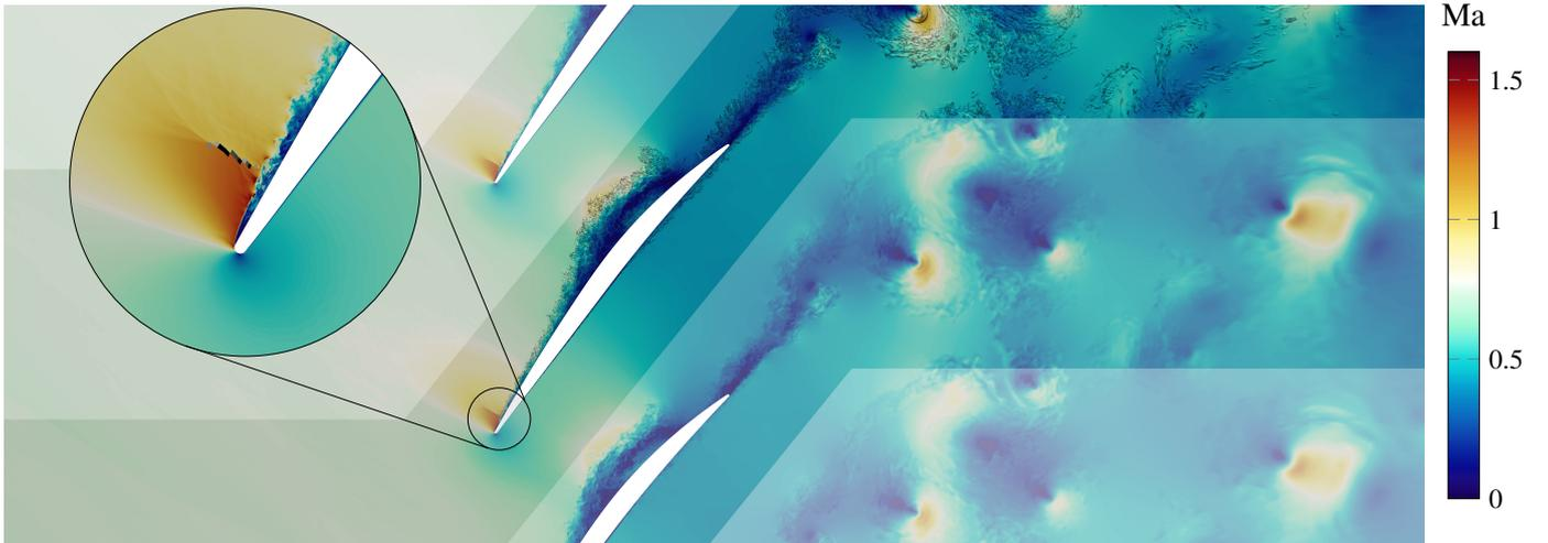
Figure 13: Instantaneous field solution for the NASA Rotor 37 case colored by the Mach number. A zoom of the leading edge highlights the supersonic flow region with the local blending values  $\alpha$  of the FV shock capturing scheme overlaid for all elements with  $\alpha = 0.1$  (light gray) up to  $\alpha = 0.7$  (black). The domain is periodically extended which is indicated by a blurred overlay.
