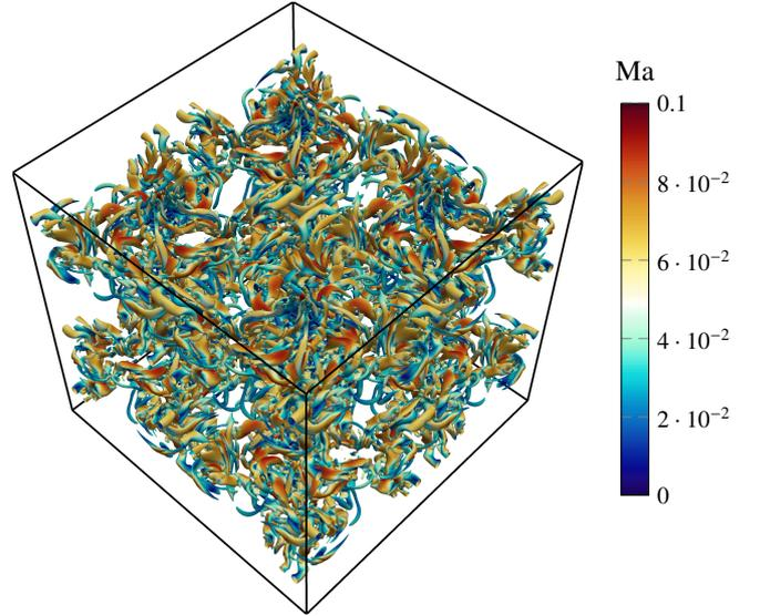
Figure 10: Instantaneous flow field of the incompressible TGV case with  $\text{Ma}_0 = 0.1$  and  $\text{Re} = 1600$  at time  $t = 10$  using  $512^3$  DOF visualized by iso-surfaces of the Q-criterion colored by Ma.
