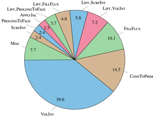
Figure 5: Portion of compute time in percent for individual routines on HAWK-AI with  $N = 7$ , split-form DG and  $8.9 \times 10^5$  DOF on a single GPU. Routines associated with the computation of the gradients via the lifting method are prefixed with “LIFT.”. Various small routines associated with performing the actual time integration, i.e. updating  $U$ , are summarized under Misc.
