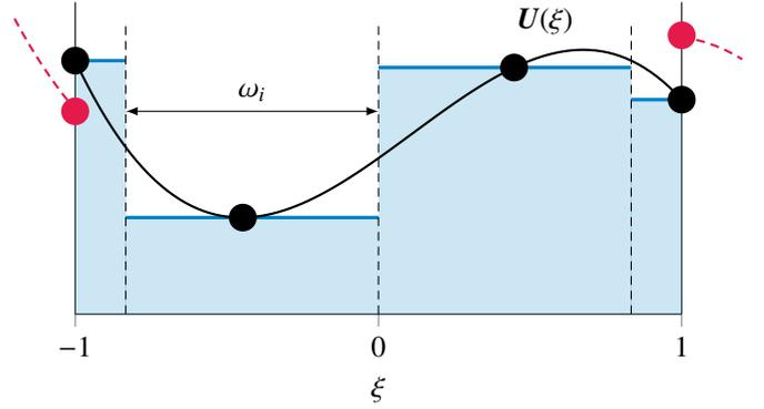
Figure 2: Sketch of the sub-cell shock capturing scheme. The DG polynomial using LGL points and a polynomial degree of  $N = 3$  is shown in black with the interpolation points indicated as dots and the integral mean solution within the subcells is shown in blue. The solution in the neighboring DG elements is indicated in red.
