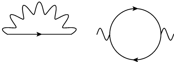
FIG. 1. Self-consistent one-loop electron self-energy (left panel) and polarization bubble for Einstein phonon (right panel). Solid lines indicate the renormalized electronic Green's function G(k) and wavy lines the renormalized Einstein phonon propagator \chi(q) .
