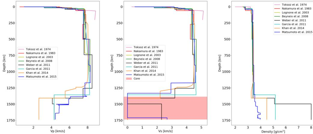
**Figure 24.** P-wave velocity (left), S-wave velocity (center), and density (right) profiles from the Moon’s surface to the core (identified in red in the middle panel) for several seismic velocity models. Data used for generating these plots are from [41]. Image taken from [10].
