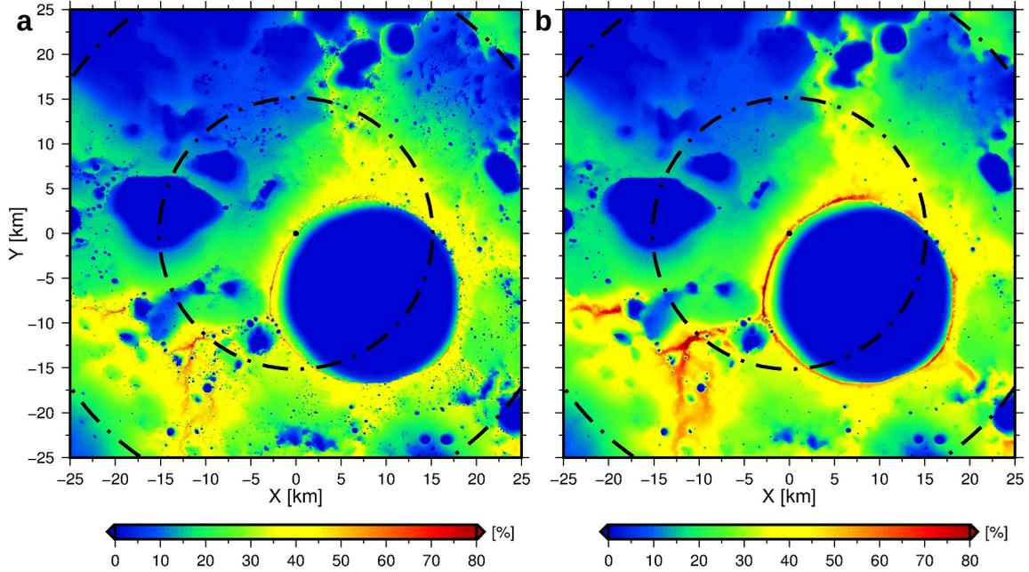
**Figure 16.** Accumulated illumination at the lunar south pole calculated over a twenty-year period and one-hour intervals. Illumination is color-coded where dark blue refers to PSRs and dark red refers to extensively illuminated spots. **a:** Accumulated illumination at the lunar surface. **b:** Accumulated illumination for an observer at two meters above the ground. Figure adapted from [101].
