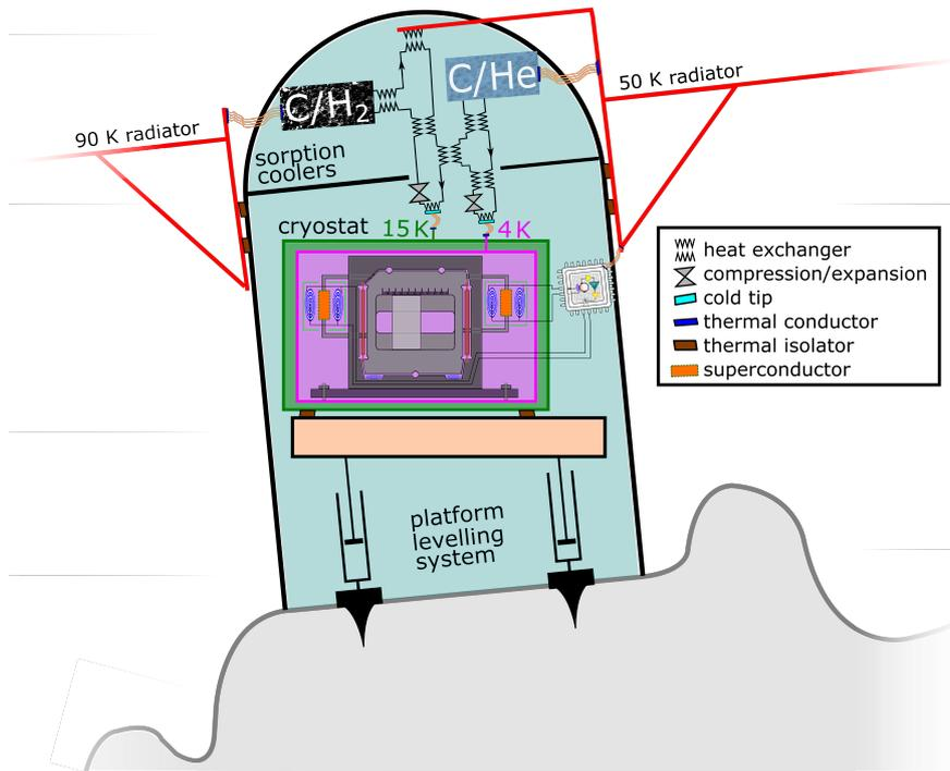
**Figure 1.** Conceptual overview of an LGWA seismic station on a tilted surface on the lunar regolith. The roughness and tilt of the lunar surface are exaggerated for illustrative purposes. Several subsystems vital to successful operation are depicted and further detailed in the text. Subsystems are not shown to scale. Figure adjusted from [20].
