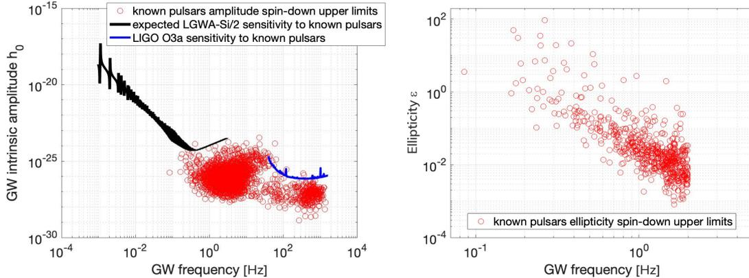
**Figure 28.** Lines: smallest detectable signal from known pulsars assuming 1 year of observation time. Circles: spin-down upper limits for known pulsars. The left plot shows the intrinsic GW amplitude, whereas the right plot the ellipticity associated with the spin-down limits.
