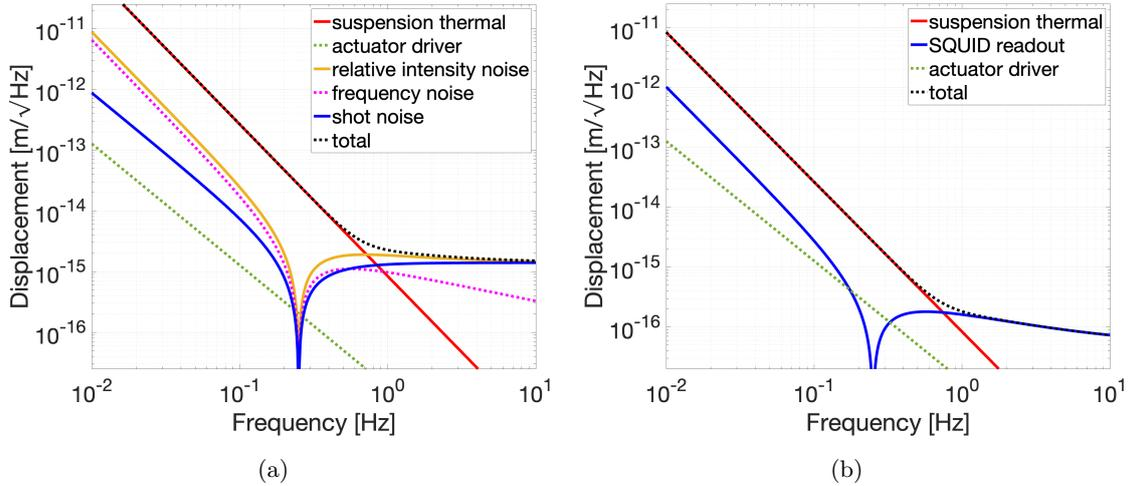
**Figure 2.** Minimum detectable inertial displacement for the two LGWA concepts: (a) a niobium Watt’s linkage with laser-interferometric readout and (b) a silicon Watt’s linkage with superconductive readout. All readout noises are corrected by the mechanical transfer function of the proof mass suspension.
