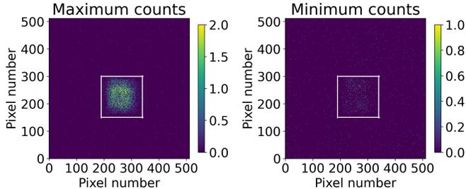
Figure S1. The background-subtracted detector images that depict the highest and lowest intensity levels in a single period of oscillation on the Anger camera [41]. The neutrons were counted only in the direct beam region of interest (ROI) outlined by the white squares with edges 150 pixels in length ( $\sim 3.5 \text{ cm}^2$ ). To convert to relative intensity used in Figs. 3 and S3, the maximum and minimum counts in the ROI were added together:  $N_0 = 8600$ .
