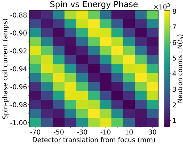
Figure 2. Relative intensities collected at specific detector translation positions and scanned through the spin-phase  $\alpha$  at each detector position  $\delta$  relative to the MIEZE focusing condition [see Eq. (13)], which is proportional to the energy phase  $\gamma$  [see Eq. (14)]. The frequencies of RF1 and RF2 were set at 45 kHz and 50 kHz, respectively. Negative values represent translation away from the analyzer.
