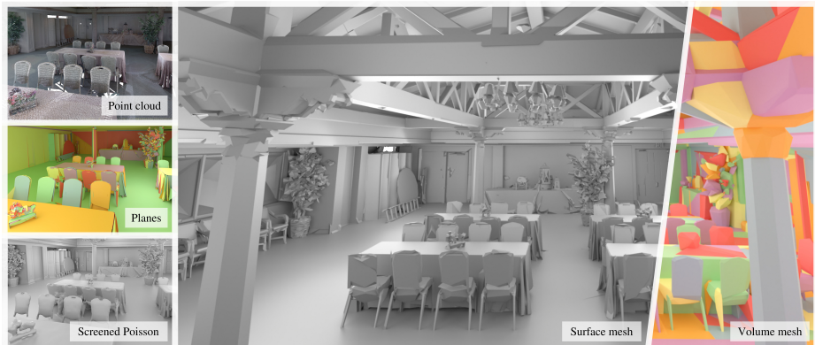
Fig. 1: Our representation of the Meeting Room [18] as a watertight and intersection-free surface mesh with 90k polygonal facets (center) or as a simplified volume mesh with 2500 convex polyhedra (right). Our method inputs 40k planes (middle left) detected from a LiDAR scan of the scene (top left). For comparison, a Screened Poisson [17] reconstruction consists of over 6M triangles (bottom left).
