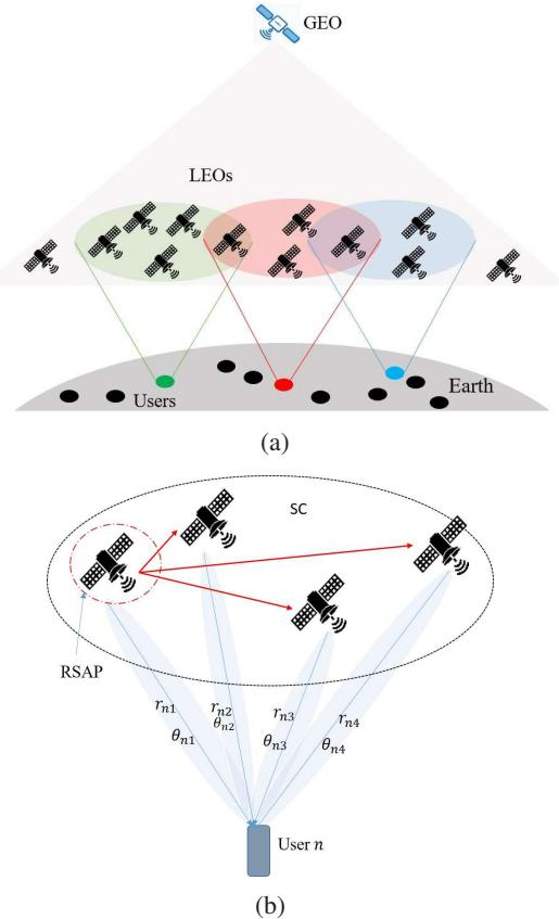
Fig. 1: UC-DMIMO system in space. a) general system with a GEO satellite working as a CPU and a set of orbiting LEO satellites working as access points that jointly serve ground users; and b) the  $n$ -th SC of LEO satellites selected based on a user-centric clustering approach and cooperatively work as a distributed antenna system to serve the  $n$ -th user.
