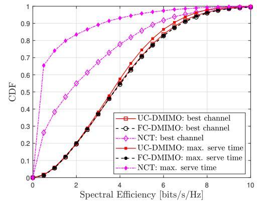
Fig. 3: Comparison of the downlink per-user spectral efficiency for the proposed UC-DMIMO system with the FC-DMIMO and the NCT when the RSAP is selected based on the best channel and based on the maximum service time.
