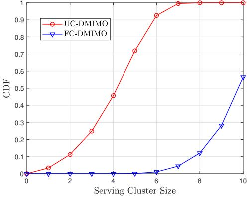
Fig. 4: User's SC size for the proposed US-DMIMO compared with that of FC-DMIMO when the RSAP is selected based on the best channel.
