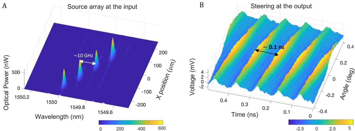
FIG. 2. (A) Spectra measured in the Fourier plane of the VIPA indicating a frequency gradient array of four comb lines each spatially resolved. The comb lines are separated by 9.8 GHz in frequency and by  $\sim 153$   $\mu\text{m}$  in space. (B) Measured temporal waveforms from Spatial Fourier transform of (A) reveal full-duty-cycle continuous beam steering over an angular range of  $0.8^\circ$ . The steering repeats every  $\sim 101$  ps consistent with the frequency spacing of the comb lines.
