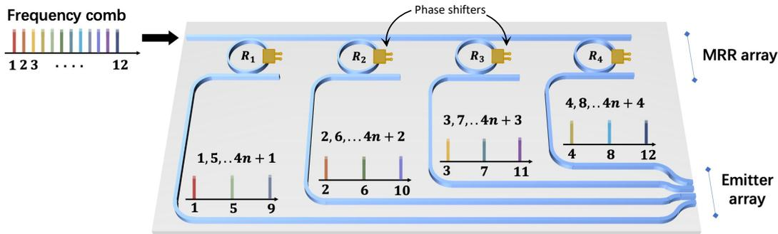
FIG. 4. Illustration of an on-chip implementation design to realize a frequency gradient array for full-duty cycle beam steering. The design features a microring filter array used to select desired set of comb lines from the input comb that are subsequently routed to emitters.
