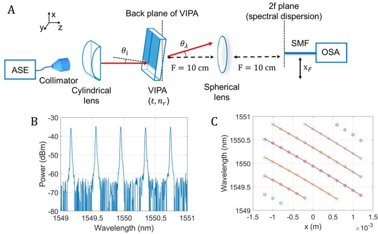
Fig. S1. (A) Experimental setup for VIPA characterization. ASE: Amplified spontaneous emission, VIPA: Virtually imaged phased array, SMF: Single-mode fiber, OSA: Optical spectrum analyser. (B) Spectrum measured at one spatial location in the Fourier plane of VIPA. (C) Dispersion data from measurements in the Fourier plane of the VIPA resulting in a fitted incident angle of  $7.56^\circ$ .
