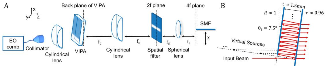
Fig. S3. (A) Experimental setup. MLL: mode-locked laser, VIPA: virtually imaged phased array, SMF: single-mode fiber. (B) VIPA structure, virtual sources, and multiple reflections within the VIPA.
