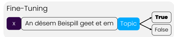
(a) The model is fine-tuned on detecting whether a topic is present in a sample x or not (= binary classifier). Translation: This example is about...
