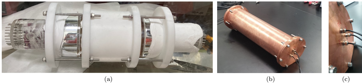
FIG. 5. Picture of 4-inch length crystal assembly. (a) Inner structure of 4-inch long crystal and PMTs assembly. (b) Encapsulated detector with copper case and cable grands. (c) Zoomed picture of cable grands to secure detector.
