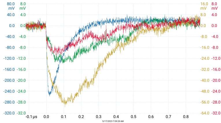
Figure 2: The typical waveforms: the blue curve corresponds to the plastic scintillator tile, while the green, yellow, and red curves correspond to the glass scintillator tiles.
