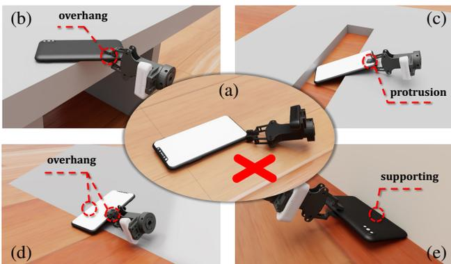
Fig. 2: **Pre-grasping leverages environmental features to enhance graspability.** (a) An object lying flat on the floor, ungraspable in its current position. (b) Side-grasping an object that overhangs a surface. (c) Grasping an angled part protruding from a slot. (d) Grasping the middle of a phone suspended at the foot of a slope. (e) Pinning a phone against a wall and grasping it from the opposite side.
