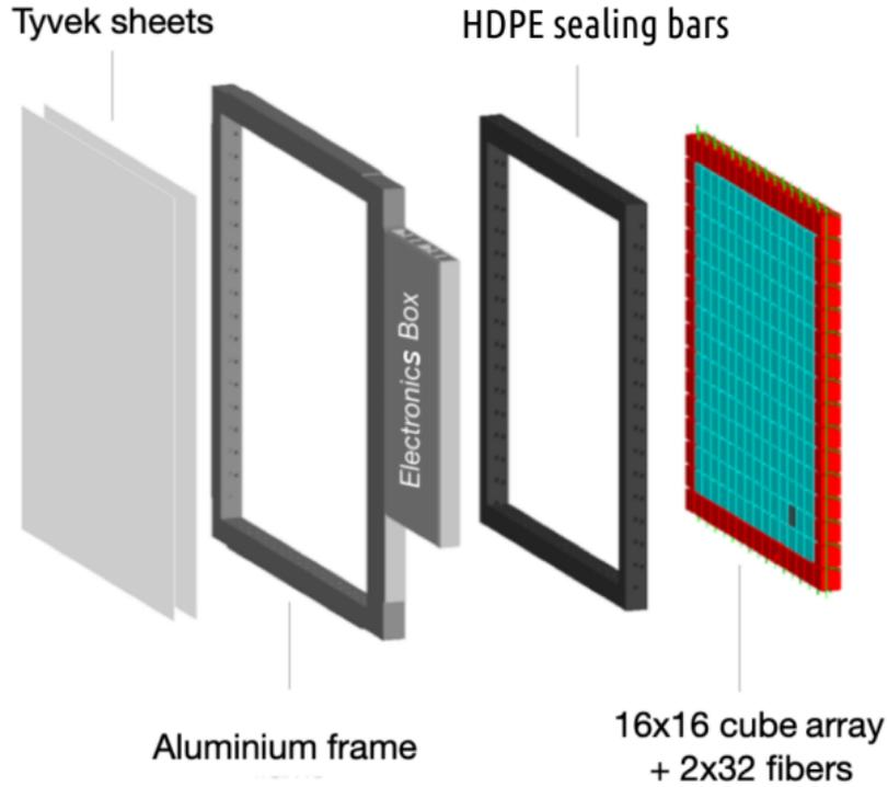
Figure 1: The composition of the SoLid detection plane.
