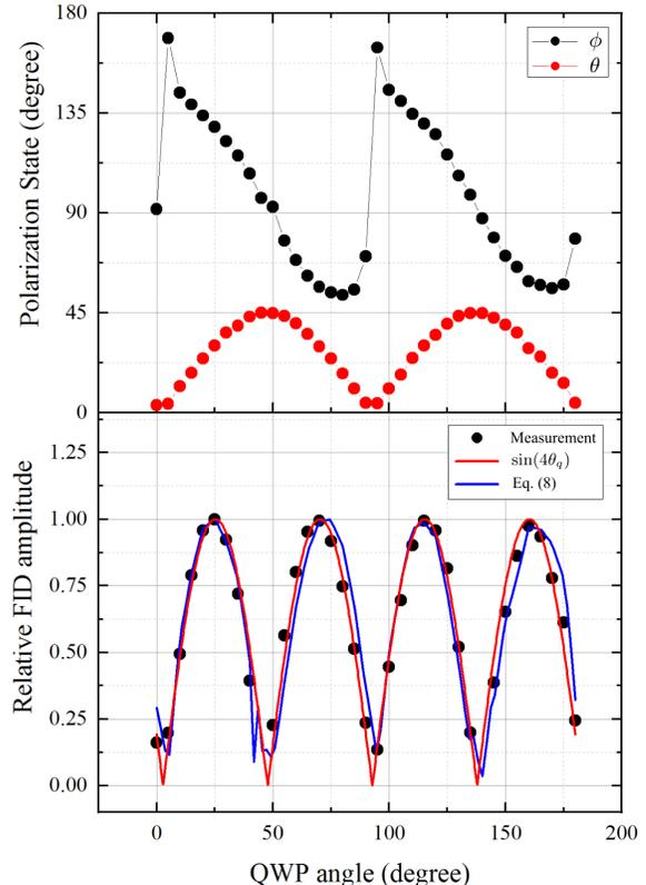
FIG. 7. The polarization state of incident beam(upper plot) and relative FID amplitude(bottom plot) as a function of QWP angle. When the QWP angle is  $25^\circ$  where relative FID amplitude is maximized,  $\theta$  is  $30^\circ$  and  $\phi$  is  $129^\circ$ . The red line shows  $\sin(4\theta_q)$  behavior to the QWP angle  $\theta_q$ . Blue line illustrates Eq. (8) calculated based on the polarization state on the top plot.
