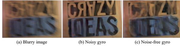
**Fig. 9:** Effect of training with noisy gyro data. (a) Real-world blurred image. (b) Model trained with noisy gyro data. (c) Model trained with noise-free gyro data.
