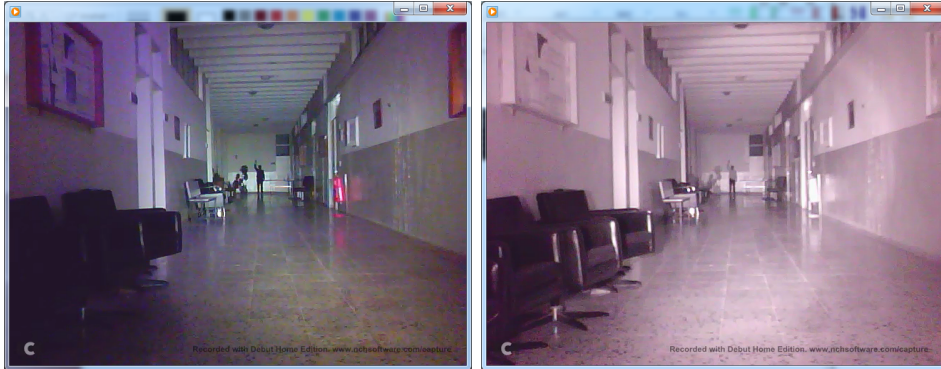
Fig. 8. Two photographs of a 50 m long and completely dark corridor taken by a webcam after illuminating by the projector with white LED (left) and with IR LED (right).
