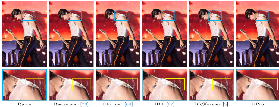
Fig. 9: Qualitative comparisons with state-of-the-art methods on Internet-Data [62] for real rain removal. (Zoom in for a better view.)
