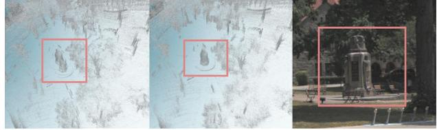
Figure 3. **Sequence alignment visualization.** The initial GPS-based alignment is imprecise, as evidenced by the duplicated structures in the overlaid LiDAR point clouds (left). After our ICP alignment, the area is well reconstructed (middle) according to its real geometry (right, from Argoverse 2 [64]).
