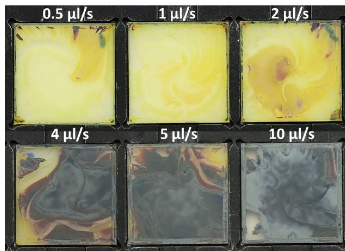
Fig. S6 Photographs of perovskite thin films produced with different dispense speeds of organic ammonium salt. The speeds are 0.5, 1, 2, 4, and 5 \mu\text{l/s} , respectively.
