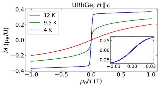
FIG. 1. (color online) Magnetization  $M$  of URhGe measured with  $H \parallel c$ . The inset is an enlarged view of the 4.0-K data around  $H = 0$ . Below  $T_C$ ,  $M(H)$  exhibits step-function like behavior with a narrow hysteresis, indicating that the multi-domain state is almost negligible.
