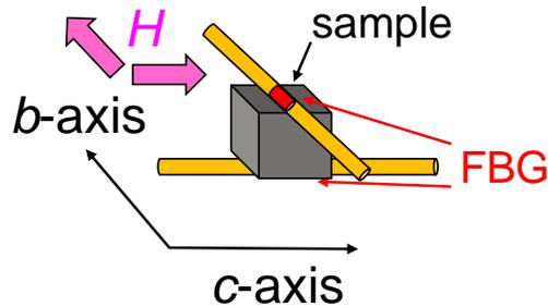
FIG. S1. Schematic to explain how to paste FBG sensors to the sample. We pasted two FBGs parallel to the  $b$  and  $c$  axes of the sample, respectively, in order to perform multi-axis simultaneous strain measurements. We performed two sets of experiments with the applied magnetic field along either the  $b$  or  $c$  axis.
