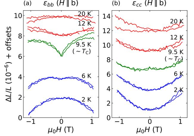
FIG. 3. (color online) Magnetostriction of URhGe in (a)  $\varepsilon_{bb}$  and (b)  $\varepsilon_{cc}$  measured under  $H \parallel b$ . Each curve is vertically offset for clarity. V-shaped magnetostriction was not observed below  $T_C$  (blue curves), whereas the behavior above  $T_C$  (red curves) and at  $T_C$  (green curves) qualitatively resembles those observed under  $H \parallel c$  (Fig. 2).
