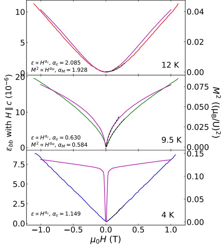
FIG. S3. Comparison of  $\epsilon_{bb}(H)$  (red, green, blue curves; left axis) and  $M^2(H)$  (purple curves; right axis) of URhGe measured under  $H \parallel c$  at various temperatures.
