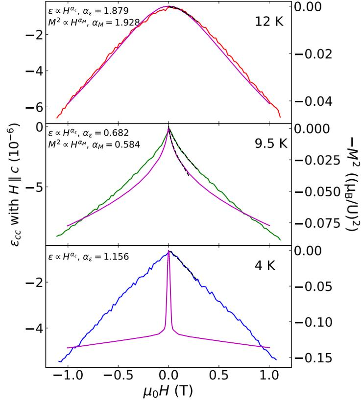
FIG. S4. Comparison of  $\epsilon_{cc}(H)$  (red, green, blue curves; left axis) and  $-M^2(H)$  (purple curves; right axis) of URhGe measured under  $H \parallel c$  at various temperatures.
