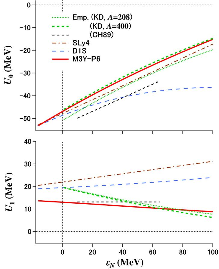
FIG. 1. Energy dependence of  $U_0$  and  $U_1$  for homogeneous nuclear matter [see Eq. (7)] at  $\rho = 0.16 \text{ fm}^{-3}$ . The s.p. potentials given by the SCMF interactions, Skyrme-SLy4 (brown dot-dashed lines), Gogny-D1S (blue long-dashed lines) and M3Y-P6 (red solid lines), are compared with the empirical potentials, KD evaluated at  $A = 208$  (green dotted lines), at  $A = 400$  (green short-dashed lines) and CH89 (black short-dashed lines).
