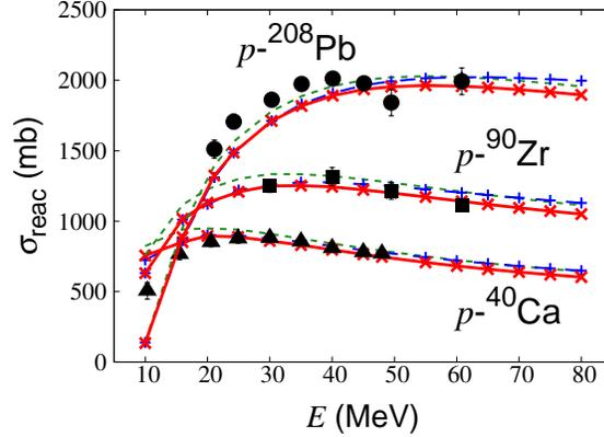
FIG. 3.  $\sigma_{\text{reac}}$  of  $p$ - $^{40}\text{Ca}$ ,  $p$ - $^{90}\text{Zr}$  and  $p$ - $^{208}\text{Pb}$  scattering. Results of  $\mathcal{V}^{\text{SFP}}$  with M3Y-P6 (D1S) plus  $\mathcal{W}^{\text{emp}}$  are plotted by crosses connected with red solid lines (pluses with blue long-dashed lines), and those of  $\mathcal{V}^{\text{emp}}$  are displayed by green short-dashed lines. Black circles, squares and triangles are experimental data [61, 69–71].
