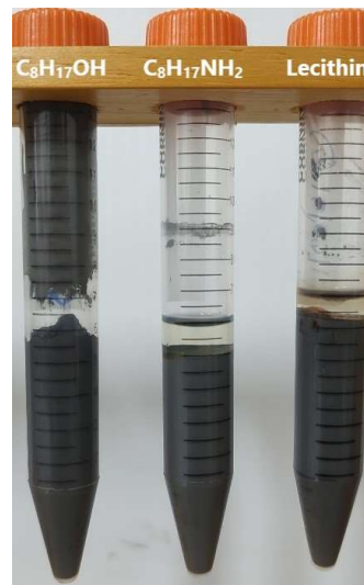
Figure 7: Picture of the test tubes containing MRF samples from the redispersibility test, after four years at rest. From left to right: octan-1-ol, octan-1-amine and lecithin.
