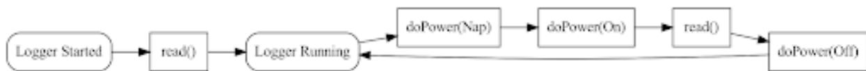
Figure 3: Illustration of the firmware routine for sensor reading and power management via modules.
