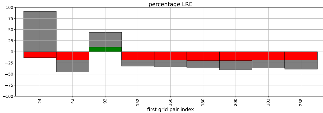
Figure 15. LRE scores for the nine grid-cell pairs with the worst MRE scores from the coarse regional study before and after the iterative refinement process; see (21) for the cell indices. Gray bars denote the initial LREs, and the green and red colored bars are the final LREs after the IR procedure with convergence tolerance of \pm 20\% . Note that the FA spectral space size is (\mathcal{N}, \mathcal{M}) = (16, 32) ; refer to the accompanying explanation for more details. See Figure 7 for more details on the LRE scores.
