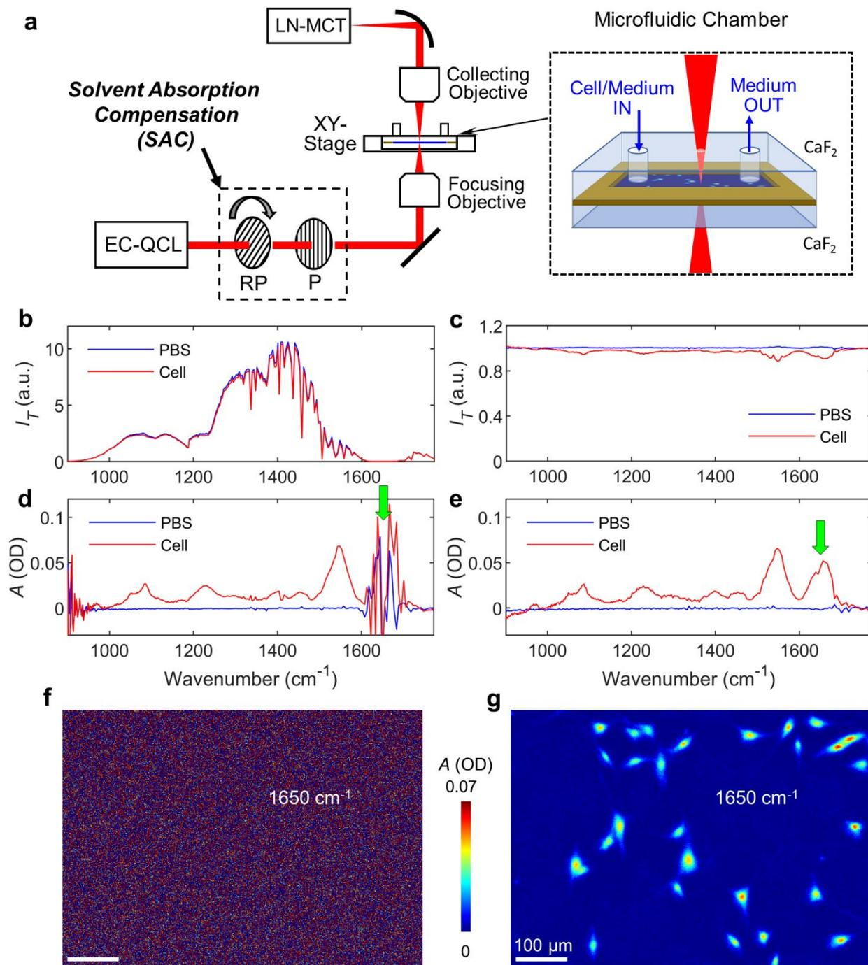
**Figure 1.** (a) Schematic of solvent absorption compensation infrared (SAC-IR) microscopy setup. The laser intensity is controlled as a function of wavelength by a pair of rotating and fixed polarizers. EC-QCL: external-cavity quantum cascade laser; RP:
