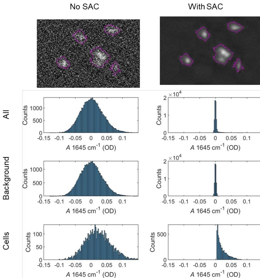
**Figure S3.** Histogram of  $1645\text{ cm}^{-1}$  absorbance values in IR absorbance images in Fig. 1d,e. An intensity threshold was used to segment absorbance images into the background and cells. The same masking areas were used for SAC and non-SAC images. The standard deviation of the background pixels was 25 mOD and 2 mOD for non-SAC and SAC images. The standard deviation of 2 mOD corresponds to the limit of detection of 0.8 mg/mL for BSA at the amide I peak.
