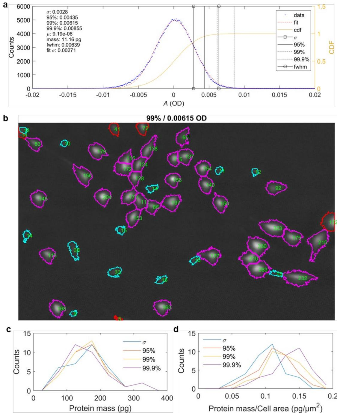
**Figure S5.** Selection of absorbance threshold level and sensitivity of threshold levels on protein mass measurements. (a) Histogram of background absorbance values from the unmasked area. The blue dots represent data; the dashed red line is a Gaussian fit; and the yellow line is the cumulative distribution function (cdf, on the right axis). The vertical lines denote the standard deviation, 95%, 99%, 99.9%, and the full-width half maximum
