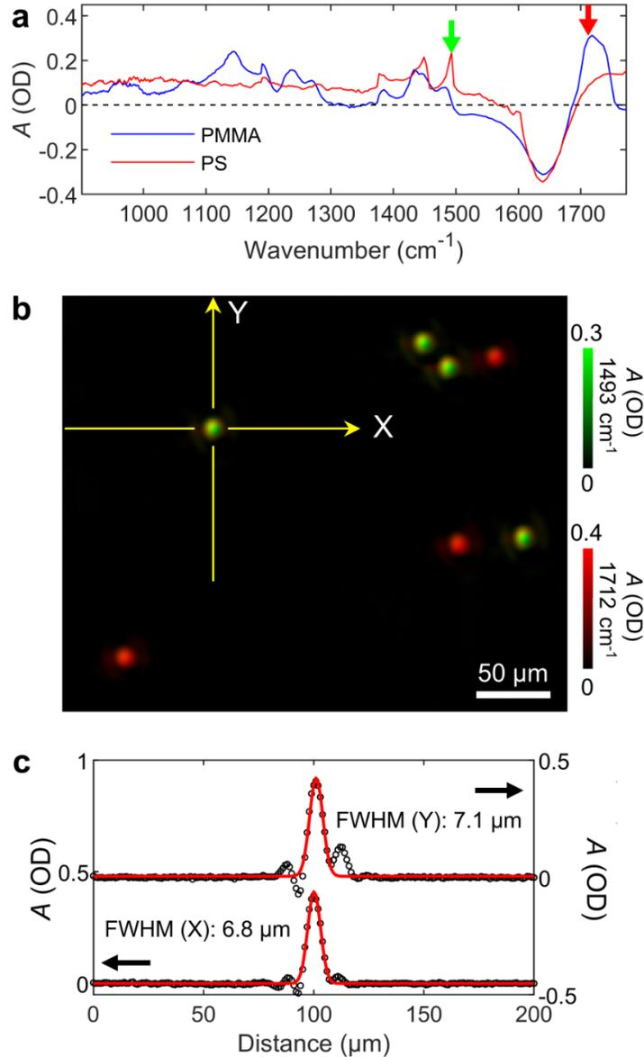
**Figure 2.** System performance using a mixture of 5- $\mu\text{m}$  diameter polystyrene (PS) and poly(methyl methacrylate) (PMMA) microparticles in water with a 25  $\mu\text{m}$  spacer. (a) IR spectra of the PS and PMMA microparticles using SAC. (b) Composite image with absorbances at 1493  $\text{cm}^{-1}$  (green) and 1712  $\text{cm}^{-1}$  (red) using SAC. (c) Line scans of the indicated PS particle in panel b.
