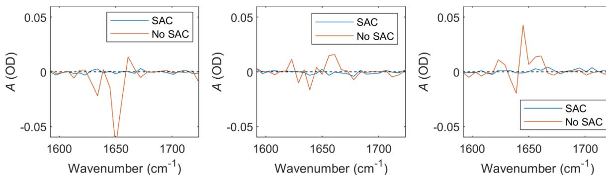
**Figure S4.** Example absorbance spectra of three single-pixel water regions with and without SAC. The dotted line is a guide to the eye and shows zero absorbance. The spectral noise was taken as the standard deviation of absorbance values in the 1623  $\text{cm}^{-1}$  – 1672  $\text{cm}^{-1}$  region. The mean spectral noise in the background region using the image mask in Figure S2 is 20 mOD and 2 mOD for non-SAC and SAC.
