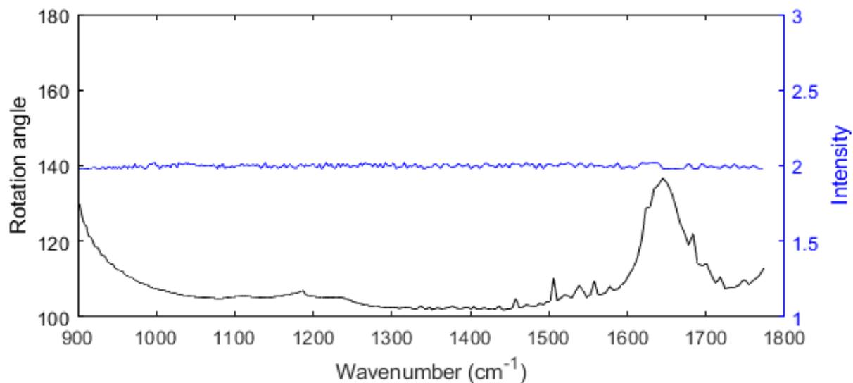
**Figure S1.** Example of polarization rotation calibration of a CaF<sub>2</sub> sample chamber filled with water with a 25  $\mu\text{m}$  spacer. The left axis (black) shows a rotation angle of the moving polarizer set to reach a setpoint LIA signal (blue, right axis).
