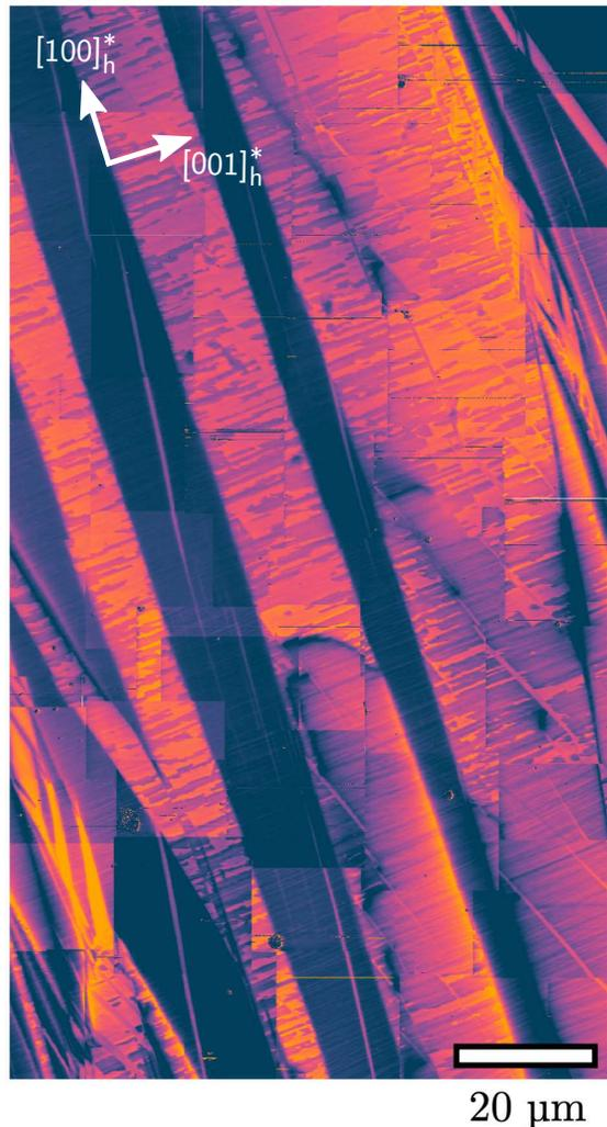
FIG. 2. Stitched MFM scans of  $\text{Fe}_7\text{S}_8$  displaying the distribution of the three types of domains revealed by applying a small magnetic out-of-plane field of 0.07 T. A clear preferential strip direction of the  $[100]_h^*$  (right to left diagonal), as expected
