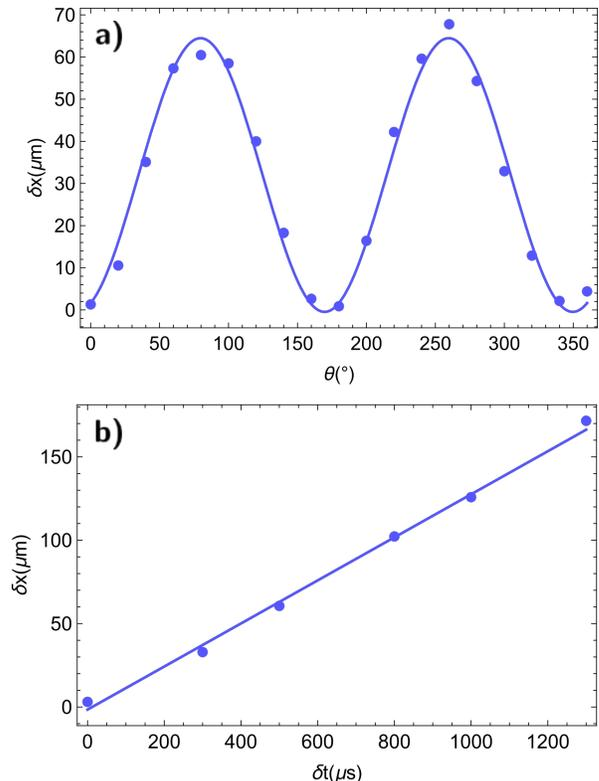
FIG. 7. Measurement of the scalar and tensorial polarizabilities: (a) Displacement  $\delta x$  of the atomic center-of-mass as a function of the angle  $\theta$  of the light polarization with respect to the magnetization axis, together with the sinusoidal fit by Eq. 3 (line). (b) Displacement  $\delta x$  of the atomic center-of-mass as a function of the laser pulse duration  $\delta t$  together with a linear fit (line).
