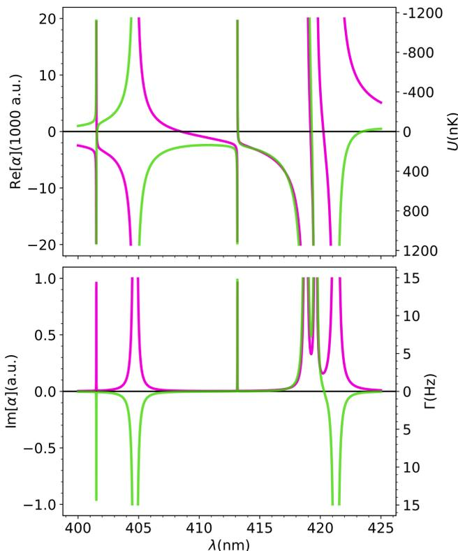
FIG. 2. Theoretical polarizability of dysprosium in the blue region. Real and imaginary part of the scalar polarizability (purple) and tensorial polarizability (green). The potential strength  $U$  and scattering rate  $\Gamma$  are calculated considering a laser power of 1 mW on a Gaussian beam with a waist of 50  $\mu\text{m}$ .
