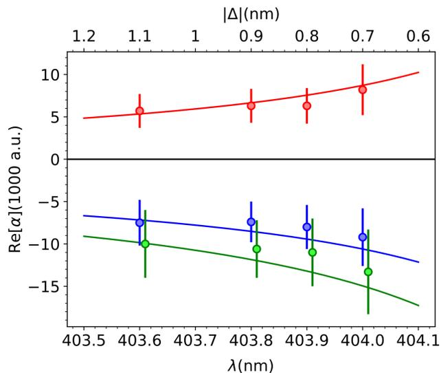
FIG. 8. Experimental polarizabilities as a function of the wavelength  $\lambda$  vs theoretical predictions. Scalar polarizability  $\alpha_s$  (blue dots), tensorial polarizability  $\alpha_t$  (red dots) and maximum polarizability  $\alpha_s - \alpha_t/2$  (green dots) show a good agreement with the theoretical predictions (lines). The green dots are shifted by 0.01 nm to the right for clarity. The upper horizontal axis indicates the detuning  $\Delta$  from the transition at 404.7 nm
