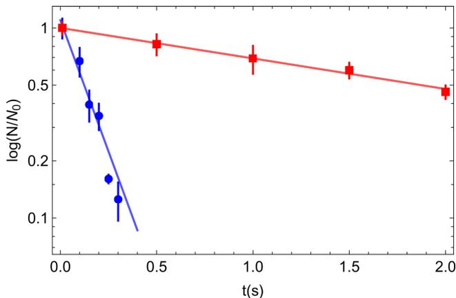
FIG. 4. Measured lifetime of a dysprosium Bose-Einstein condensate irradiated by the blue light. The lifetime with additional spectral filtering after the extended cavity (red dots) is  $(2.5 \pm 0.3)$  s, much longer than the one without (blue dots), which is  $(120 \pm 30)$  ms. Lines are exponential fits. The laser beam was Gaussian, with an average waist of  $48 \mu\text{m}$  (see text), a power of 2 mW, and a wavelength of 403.6 nm.
