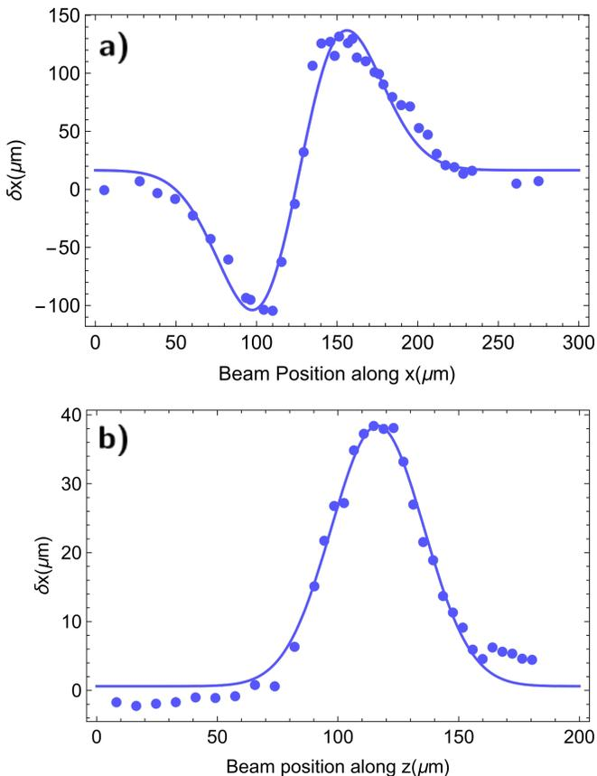
FIG. 6. Displacement measurements vs beam position. Displacement of the atomic center-of-mass  $\delta x$  on the horizontal plane as a function of the light beam position on the  $x$ -axis (a) and the  $z$ -axis (b).
