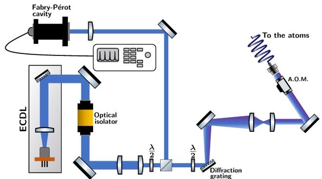
FIG. 3. Sketch of the experimental setup for the extended-cavity diode laser. The second diffraction grating, in combination with the single mode optical fiber, filters out most of the amplified spontaneous emission of the laser.
