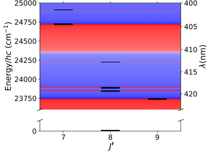
FIG. 1. Level scheme of Dy in the region of interest. Thicker black lines correspond to levels with larger linewidth. The background color scheme indicates the theoretical value of  $\text{Re}[\alpha_s - \alpha_t/2]$ , which is the value of the total polarizability shown in Eq. 3 for  $\theta = \pi/2$ . In the figure, blue (red) regions represent an overall repulsive (attractive) character.
