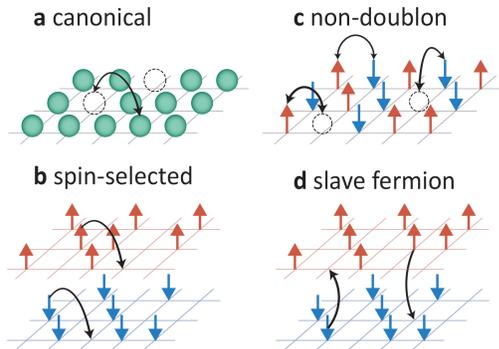
FIG. 2. **Ensemble selection via Fock-state restrictive updates.** **a** The canonical ensemble by swapping particles and holes. **b** The spin-selected ensemble by swapping particles and holes within each spin sector. **c** The non-doublon ensemble by swapping among singly-occupied electrons and holes. **d** Slave fermions by flipping the on-site spins.
