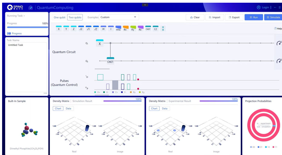
Figure 8.5: The experimental result of applying the CNOT gate pulse sequence to the state |10\rangle on SpinQ Gemini.
