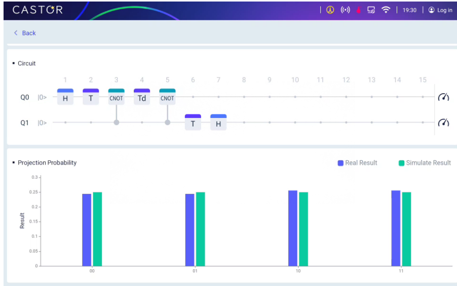
Figure 6.17: The experimental circuit and result diagram of a 2-qubit Quantum Fourier Transform on SpinQ Gemini mini.
