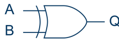
Figure 1.13: “XOR” gate Q = (A \wedge \neg B) \vee (\neg A \wedge B) = A \oplus B
