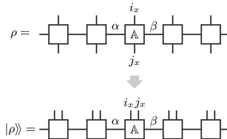
Figure 1. Matrix product density operator  $\rho$  and its corresponding doubled state  $|\rho\rangle\rangle$ . For each local tensor  $\mathbb{A}$ ,  $i_x$  and  $j_x$  denote the state in the ket and bra physical Hilbert space, respectively, and  $\alpha$  and  $\beta$  denote the state in the virtual Hilbert space.
