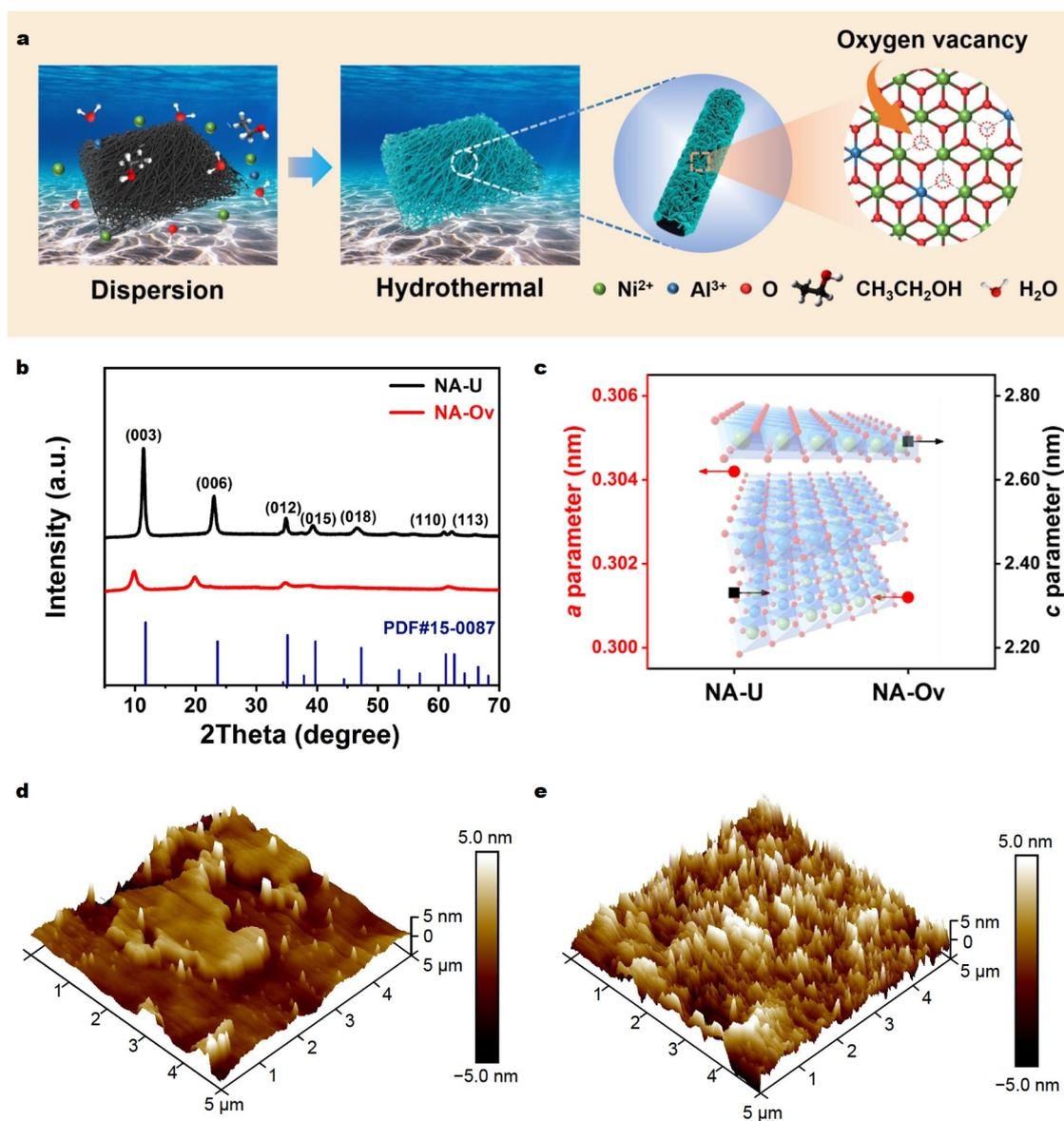
**Figure 1** (a) One-step synthesis of oxygen-deficient NiAl-LDHs/CFP electrodes. (b) XRD patterns, (c) lattice parameters of NA-U and NA-Ov. AFM 3D views of (d) NA-U and (e) NA-Ov.
