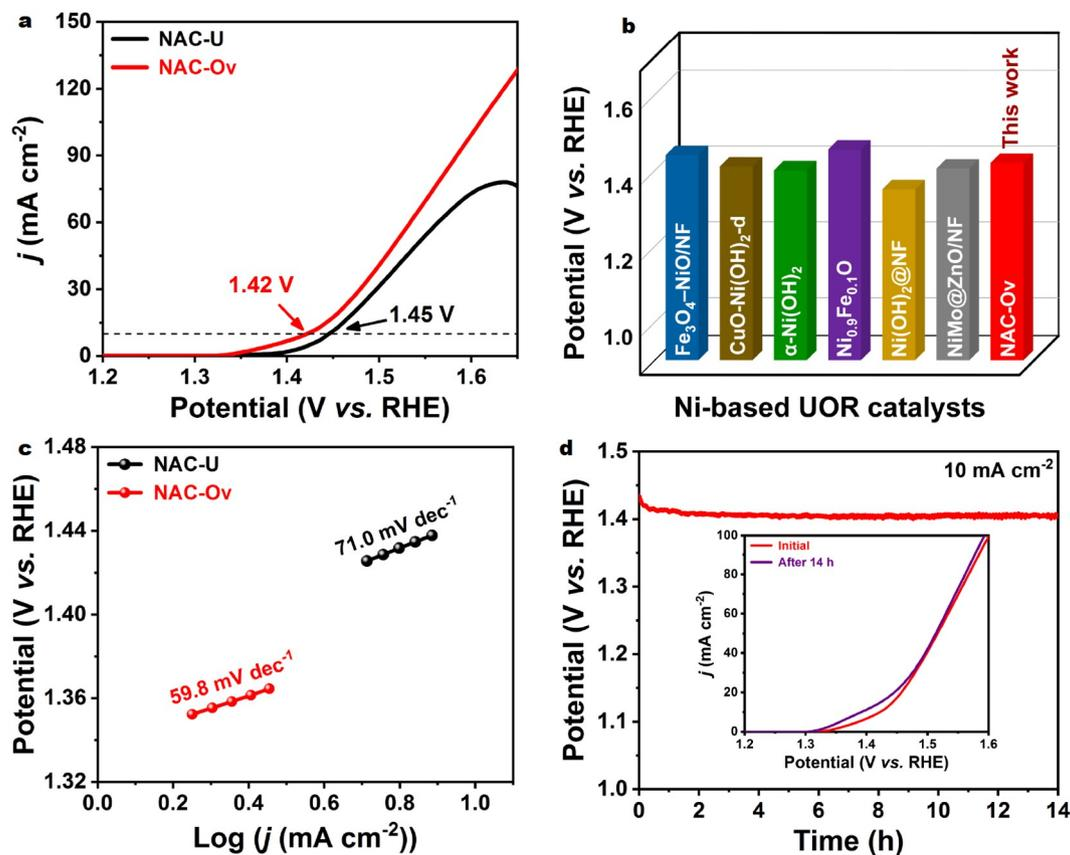
**Figure 6** (a) LSV polarization curves of NAC-U and NAC-Ov in 1 mol L<sup>-1</sup> KOH with 0.33 mol L<sup>-1</sup> urea at a scan rate of 5 mV s<sup>-1</sup>. (b) Comparison of the potential value of NAC-Ov with other nickel-based UOR electrocatalysts at a current density of 10 mA cm<sup>-2</sup>. (c) Corresponding Tafel plots. (d) CP curve of NAC-Ov at a constant current density of 10 mA cm<sup>-2</sup> for 14 h (inset: LSV polarization curves for NAC-Ov before and after CP measurements).
