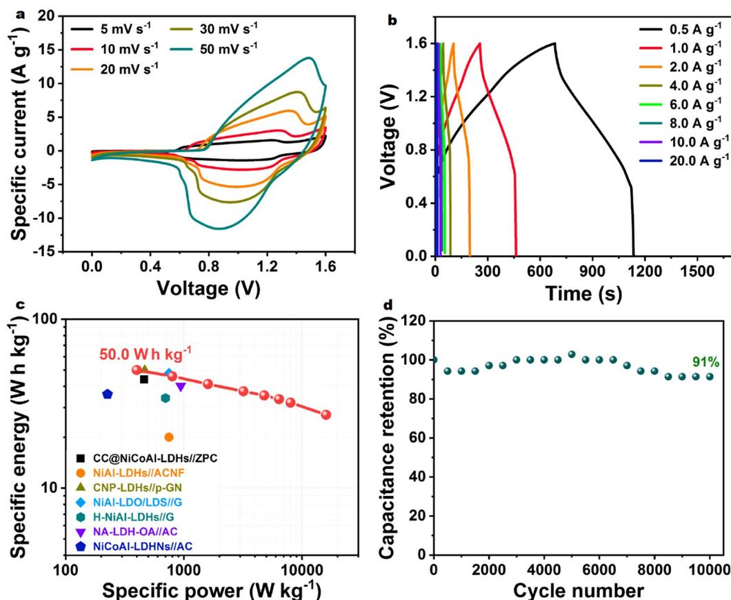
**Figure 5** (a) CV curves of the HSC at different scan rates from 5 to  $50 \text{ mV s}^{-1}$ . (b) GCD curves of the HSC at different specific currents from 0.5 to  $20.0 \text{ A g}^{-1}$ . (c) Ragone plot related to the specific energy and specific power of the HSC. (d) Cycle stability of the HSC at  $10 \text{ A g}^{-1}$ .
