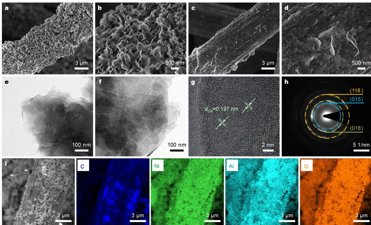
**Figure 2** FE-SEM images of (a, b) NAC-Ov and (c, d) NAC-U. TEM images of (e) NA-Ov and (f) NA-U. (g) HR-TEM and (h) the corresponding SAED images of NA-Ov. (i) EDX elemental mappings of NAC-Ov.
