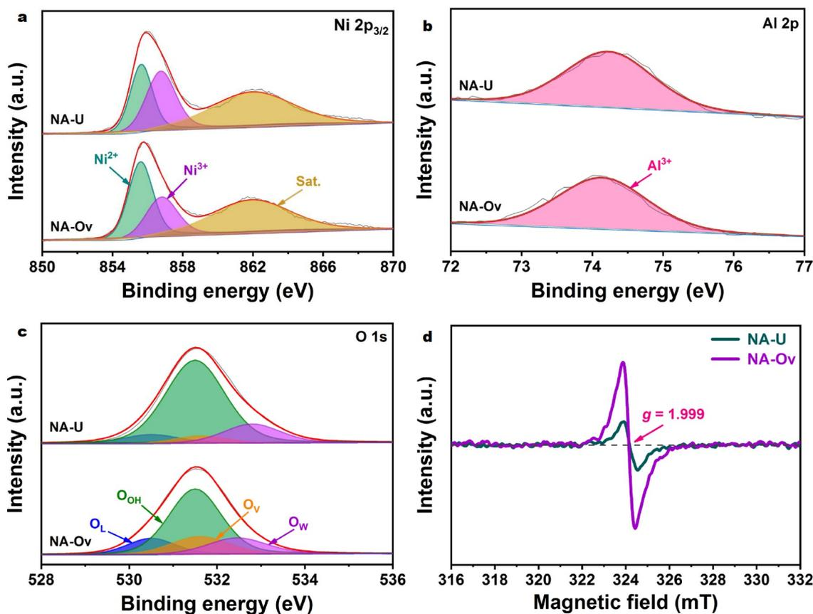
**Figure 3** XPS (a) Ni 2p spectra, (b) Al 2p spectra, (c) O 1s spectra and (d) EPR spectra of NA-U and NA-Ov.
