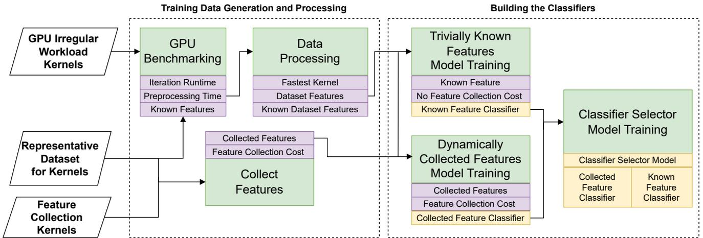
Fig. 2. Training Abstraction showing the process for training three different models. A *known features* classifier is trained on the trivially known features of the data given with the dataset. A *gathered feature* classifier is trained on statistical data that is gathered with an additional cost. Both the *known* and *gathered* data classifiers are incorporated in an *classifier selection* in which a third classifier is trained to select between the *known* and *gathered* models.
