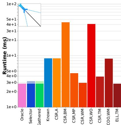
(d) **G3\_Circuit, 19 iterations**, ELL,TM is still selected as rocSPARSE has not fully amortized the preprocessing cost. Known feature predictor is incorrect and predicts that the preprocessing will be amortized at this amount of computation.
