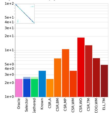
(f) **PWTK, 19 iterations**, The gathered feature based predictor is able to predict amortization, whereas the known feature predictor is unable to correctly predict that rocSPARSE preprocessing will be amortized at this number of iterations.
