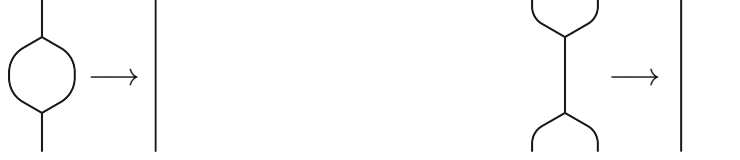
FIGURE 5. Cancellation moves of type I (left) and Type II (right). Type I moves are applied when a split contains a merge directly below it, and the two share a pair of edges. Type II moves are applied when a merge occurs directly above a split, and the two share one edge.
