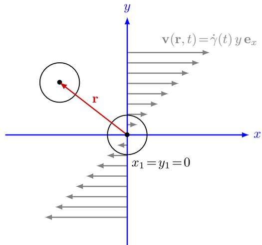
FIG. 1. Sketch of the geometry. We choose particle 1 as the origin of our cartesian coordinate system ( $\mathbf{r}_1$  is thus implicitly fixed equal to zero).
