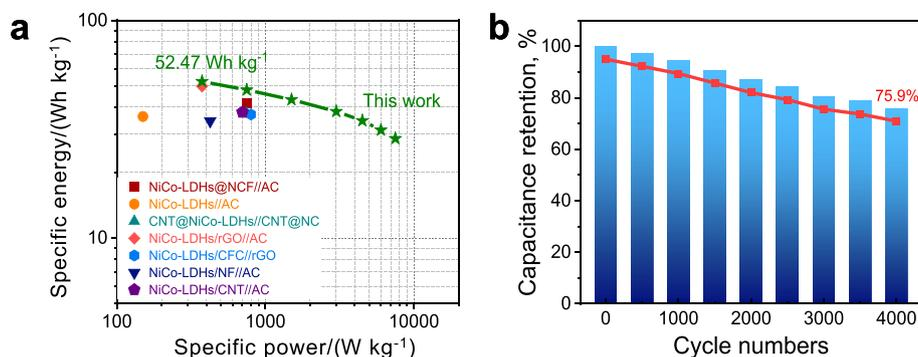
Fig. 8. (a) Ragone plot related to the specific energy and specific power of the HSC. (b) Cycle stability of the HSC at 10 A g<sup>-1</sup>.
