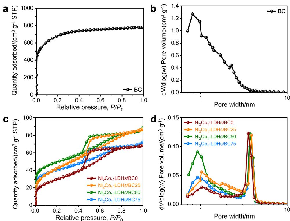
Fig. 4. (a) Nitrogen adsorption/desorption isotherm and (b) pore size distribution of BC. (c) Nitrogen adsorption/desorption isotherms and (d) pore size distribution of  $\text{Ni}_2\text{Co}_1\text{-LDHs/BC0}$ ,  $\text{Ni}_2\text{Co}_1\text{-LDHs/BC25}$ ,  $\text{Ni}_2\text{Co}_1\text{-LDHs/BC50}$ , and  $\text{Ni}_2\text{Co}_1\text{-LDHs/BC75}$ .
