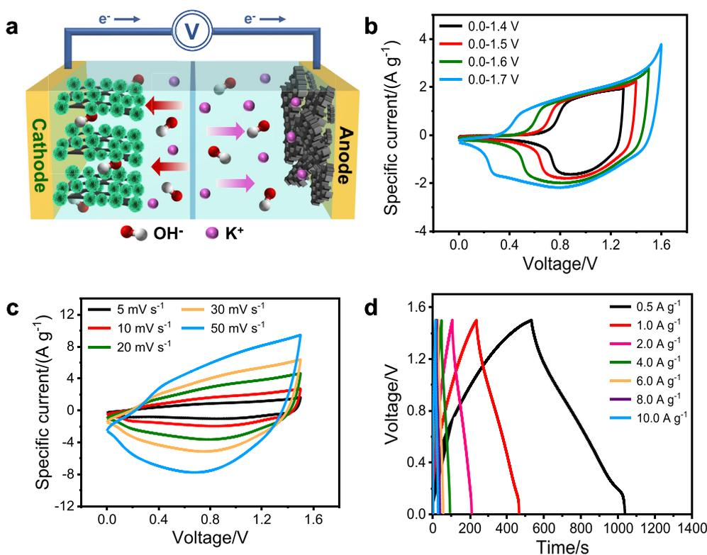
Fig. 7. (a) Schematic illustration of the as-fabricated HSC device. (b) CV curves of the HSC performed at different voltage windows at  $10 \text{ mV s}^{-1}$ . (c) CV curves of the HSC at different scan rates from  $5$  to  $50 \text{ mV s}^{-1}$ . (d) GCD curves of the HSC at different specific currents from  $0.5$  to  $10.0 \text{ A g}^{-1}$ .
