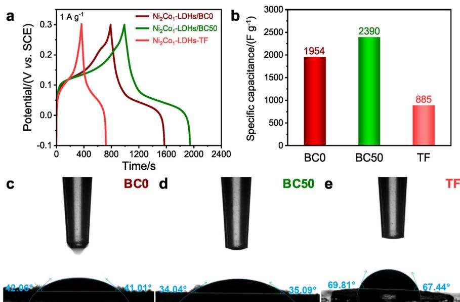
Fig. 6. (a) GCD curves and (b) corresponding specific capacitance of the  $\text{Ni}_2\text{Co}_1\text{-LDHs/BC0}$ ,  $\text{Ni}_2\text{Co}_1\text{-LDHs/BC50}$ , and  $\text{Ni}_2\text{Co}_1\text{-LDHs-TF}$  electrode at  $1 \text{ A g}^{-1}$ . Contact angle measurements of (c)  $\text{Ni}_2\text{Co}_1\text{-LDHs/BC0}$ , (d)  $\text{Ni}_2\text{Co}_1\text{-LDHs/BC50}$ , and (e)  $\text{Ni}_2\text{Co}_1\text{-LDHs-TF}$  with  $6 \text{ M KOH}$  electrolyte.
