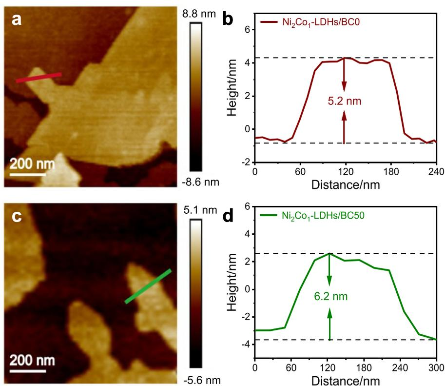
Fig. 3. AFM images and corresponding height profiles of (a, b)  $\text{Ni}_2\text{Co}_1\text{-LDHs/BC0}$  and (c, d)  $\text{Ni}_2\text{Co}_1\text{-LDHs/BC50}$ .
