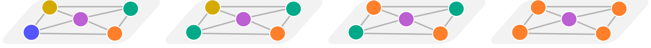
FIG. 2: Symmetry-induced pattern states. Each orbit partition induced by the graph automorphism and its subgroups creates different patterns in the network with five nodes. Four patterns are illustrated where node color corresponds to a cluster.
