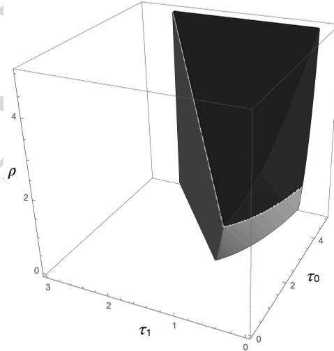
Figure 12: Domain of the space  $\{\tau_0, \tau_1, \rho\}$  where PAALs are possible  $\forall (\xi_3, \xi_1) \in \Omega$ . The darker, upper part,  $\rho > 2\tau_1$ , corresponds to  $\eta_{\max} = \eta_1$ , the lighter, lower part,  $\rho < 2\tau_1$ , to  $\eta_{\max} = \eta_2$ .
