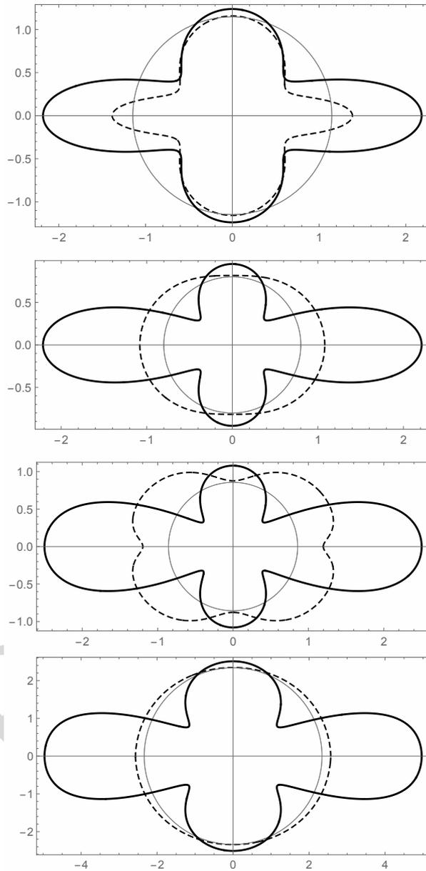
Figure 20: Directional diagrams of  $\nu_{12}$  for the four materials in Tab. 3, respectively material 1, 2, 5 and 15 from top to bottom. The dashed line is  $\nu_{12}$  of the ply. The thin circle marks the zero value: inside it,  $\nu_{12}$  is negative.
