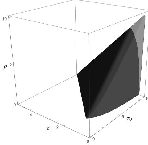
Figure 10: Domain of the space  $\{\tau_0, \tau_1, \rho\}$  where TAALs are possible  $\forall(\xi_3, \xi_1) \in \Omega$ . The exterior, light and transparent, domain corresponds to materials with  $K = 0$  and surrounds the, darker, part of materials with  $K = 1$ .
