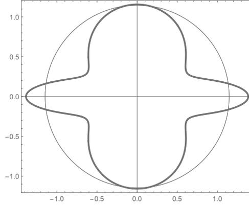
Figure 1: The directional diagram of  $\nu_{12}$  for pine wood in a plane-stress state (material data in Tab. 1, source Lekhnitskii [12]). The thin circle marks the zero value: inside it,  $\nu_{12}$  is negative.
