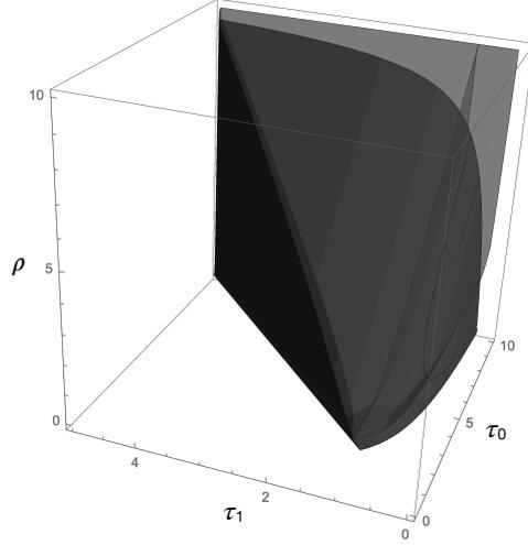
Figure 11: Domain of the space  $\{\tau_0, \tau_1, \rho\}$  where TAALs are possible for some  $(\xi_3, \xi_1) \in \Omega$ . The exterior, light and transparent, domain corresponds to materials with  $K = 0$  and surrounds the, darker, part of materials with  $K = 1$ .
