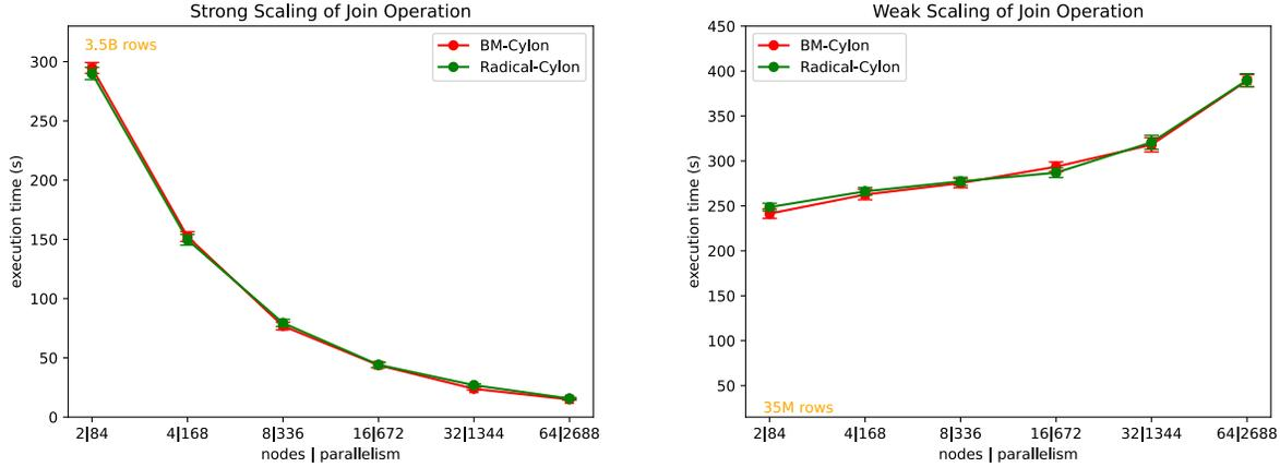
**Fig. 6.** Comparison of strong scaling(left) and weak scaling(right) performance of Bare-Metal and Radical-Cylon with join operation on *ORNL-Summit*. execution time (s) is calculated by running the task for 10 iterations and it's used for a higher scalability test. The number of parallelism is calculated by nodes multiple by 42 cores per node.
