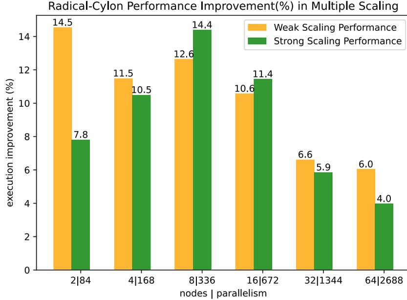
**Fig. 11.** Radical-Cylon performance improvement with scaling operation on *ORNL-Summit*. The number of nodes for batch execution is generated by the requested resource as the system allocates resources separately
