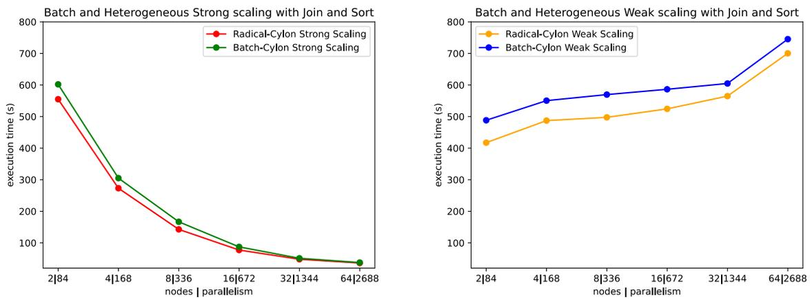
**Fig. 10.** Comparison of strong scaling(left) and weak scaling(right) performance of Heterogeneous and Batch executions on *ORNL-Summit*. execution time(s) is calculated by running task for 10 iterations. Batch execution time for join and sort is calculated separately from two batch outputs
