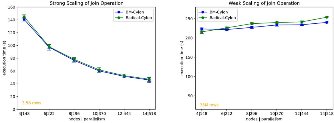
**Fig. 5.** Comparison of strong scaling(left) and weak scaling(right) performance of Bare-Metal and Radical-Cylon with join operation on *Rivanna*. execution time (s) is calculated by running task for 10 iterations. The number of parallelism is calculated by nodes multiple by 37 cores per node
