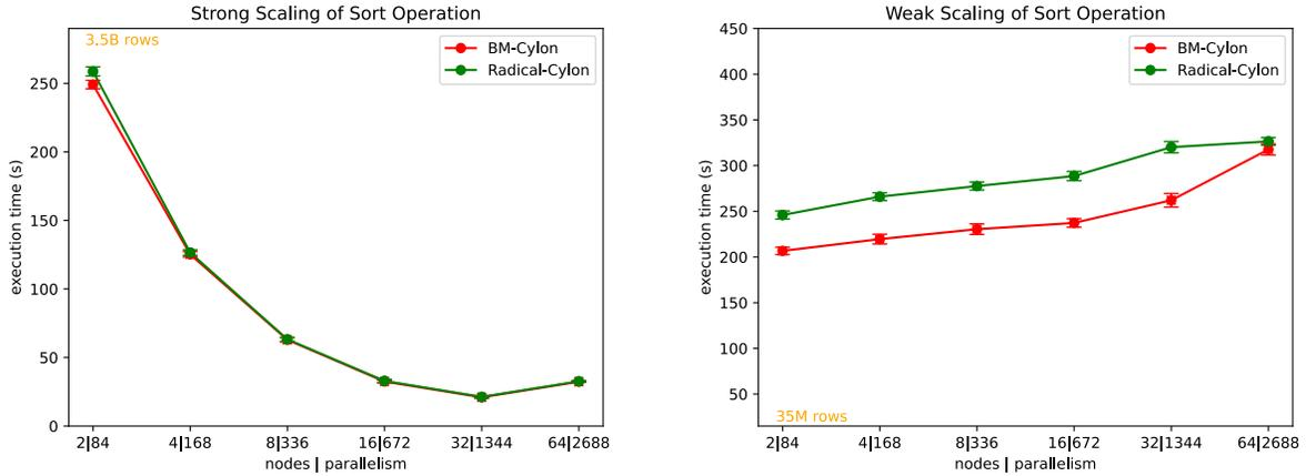
**Fig. 8.** Comparison of strong scaling(left) and weak scaling(right) performance of Bare-Metal and Radical-Cylon with sort operation on *ORNL-Summit*. The number of parallelism is calculated by nodes multiple by 42 cores per node. Strong scaling with 2688 nodes takes a bit more time than with 1344 due to the lack of rows available for each worker and some workers go idle.
