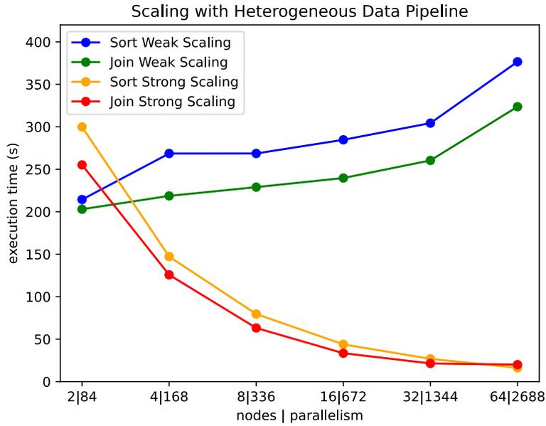
**Fig. 9.** Heterogeneous Executions with sort and join strong and weak scaling(4) operations on *ORNL-Summit*. Strong scaling with 2688 nodes takes a bit more time than with 1344 due to the lack of rows available for each worker and some workers go idle.
