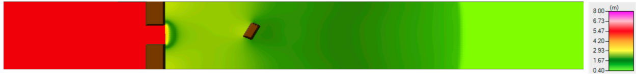
(a) Dam break HEC-RAS Simulation after 1 minute
