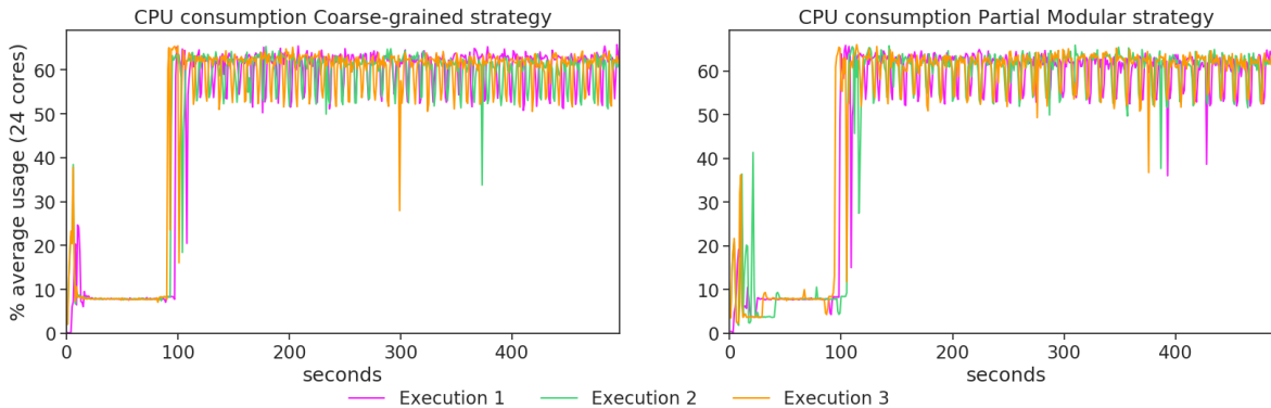
Figure 3: CPU consumption for coarse-grained and partial modular strategies.
