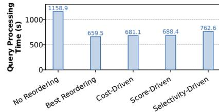
**Figure 5: Query processing time for UC1** – comparison among five system options: no reordering, best reordering, EDDY cost-driven routing, EDDY score-driven routing, and EDDY selectivity-driven routing.
