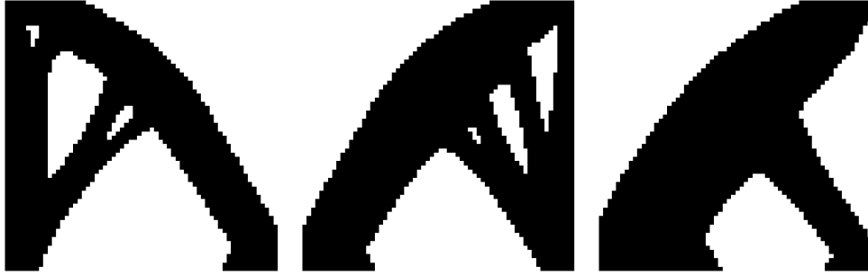
Figure 3: Three typical designs from topology optimization.
