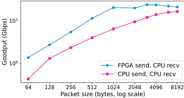
Fig. 8: Packet size vs. goodput for Beehive and Linux TCP send. The (CPU send/FPGA receive) is omitted, as it is approximately the same as (CPU send/CPU receive) due to the CPU send path being the bottleneck.
