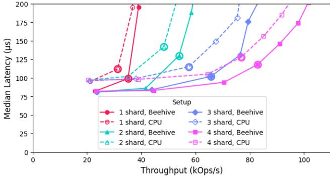
Fig. 10: Latency vs. throughput for the VR key-value store workload varying the number of shards and client threads. The FPGA witness consistently outperforms the equivalent CPU cores in both latency and throughput.
