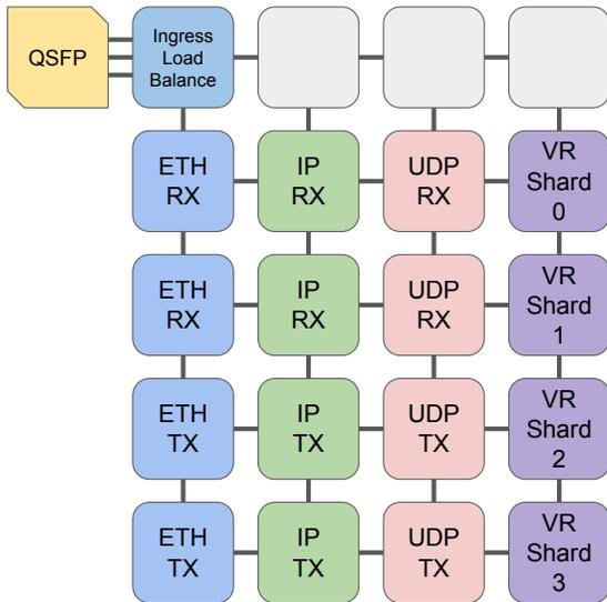
Fig. 6: Beehive tile layout for Viewstamped Replication.
