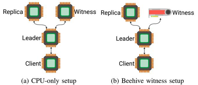
Fig. 9: Experimental setups for VR evaluation
