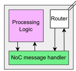
Fig. 3: Architecture of a tile.
