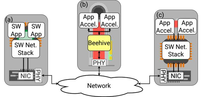
Fig. 1: (a) represents a standard CPU server node; (b) a direct-attached accelerator using the Beehive network stack; (c) an accelerator using a CPU network stack.
