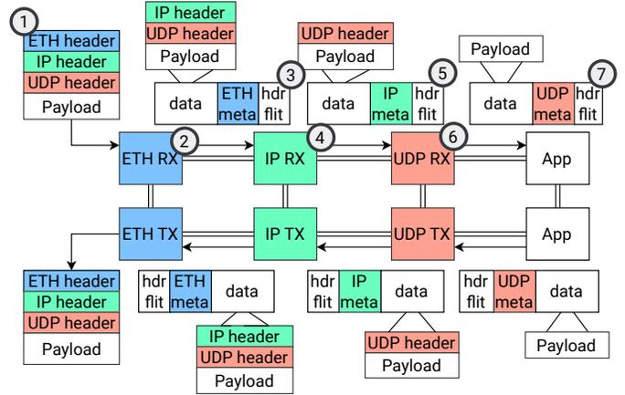
Fig. 4: The flow through which a packet is processed or constructed in Beehive.
