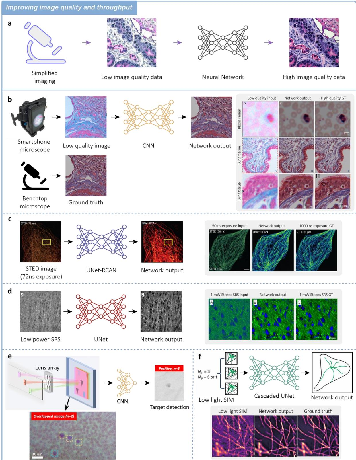
**Figure 4. Improving image quality and throughput.** **a** Schematic representation of a neural network-enabled pipeline for image quality improvement of data taken with simplified and/or inexpensive optics. **b** Deep learning enhanced mobile-phone microscopy
