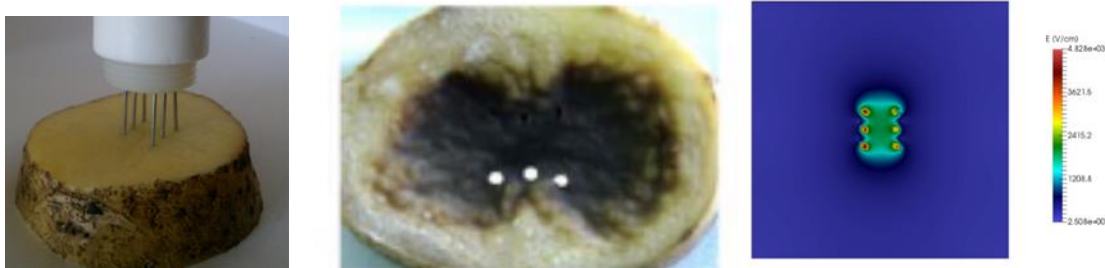
Figure 1. Experimental setup (left), the potato darkened area after the last pulse (center), simulated electric field distribution (right) for a pulse of 1500 V/cm. In the center figure, only one set of parallel electrodes is indicated by white dots. Left and center figures reproduced from [12].
